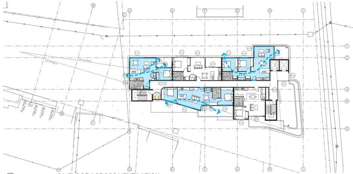
6th FLOOR | CROSS VENTILATION SCALE 1:550
