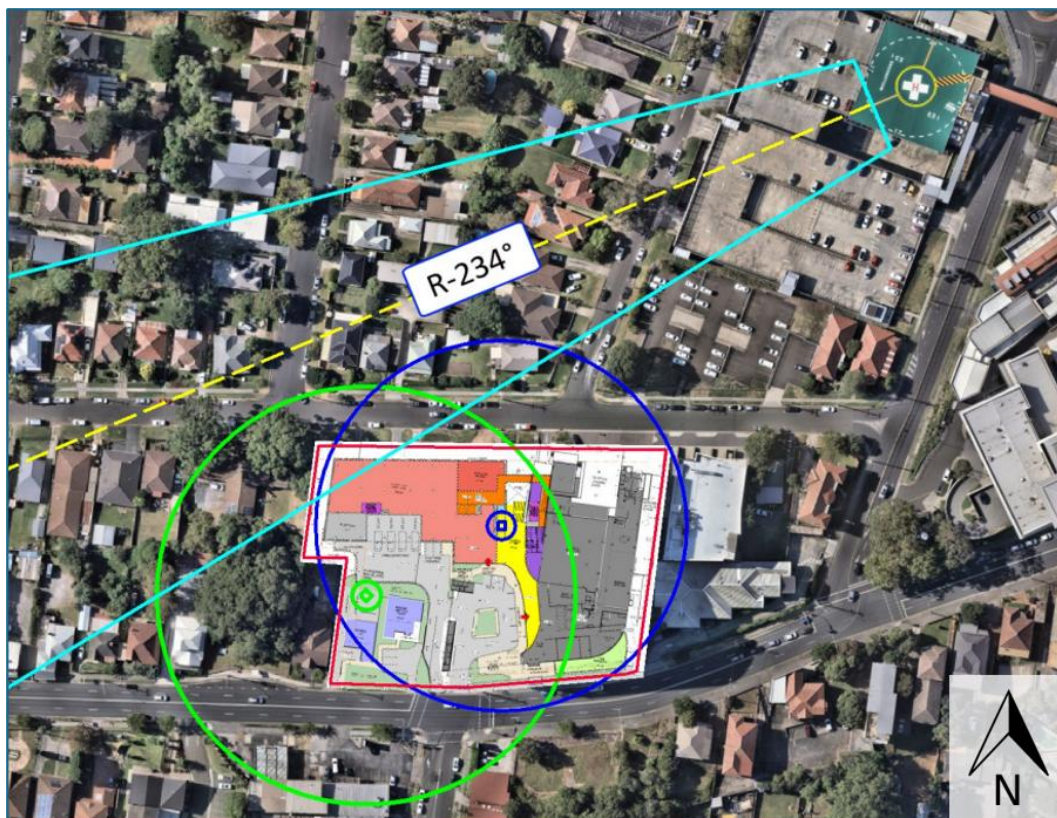
Figure 15 | Extent of intrusion into the existing operational airspace (light blue lines) from the ground level footprint and operating area for crane booms (circles) (Source: Aeronautical Impact Assessment)
