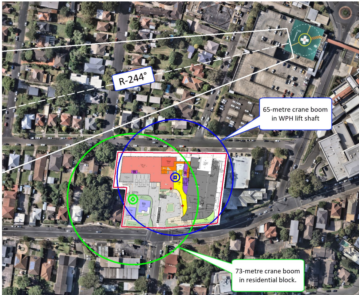
Figure 9: Operating area for construction cranes relative to the R-244° airspace
