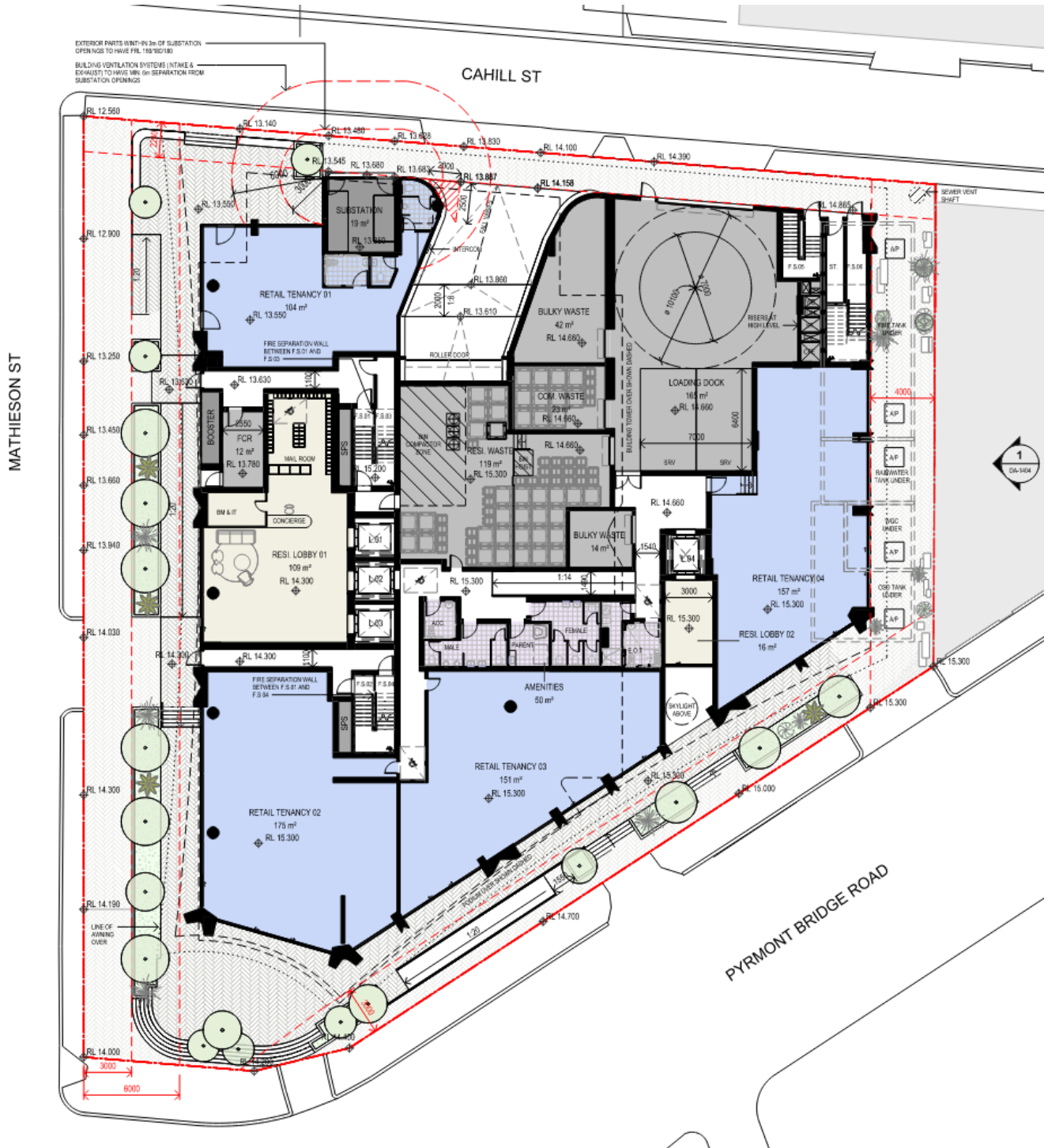
Figure 2: Architectural Plan – Ground Floor (Source: SJB Architects)
