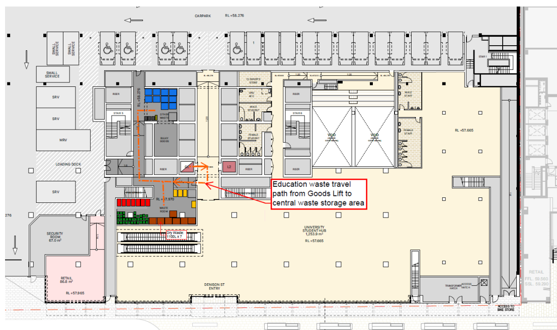
Figure 9: Waste travel from the goods lift to waste management area
