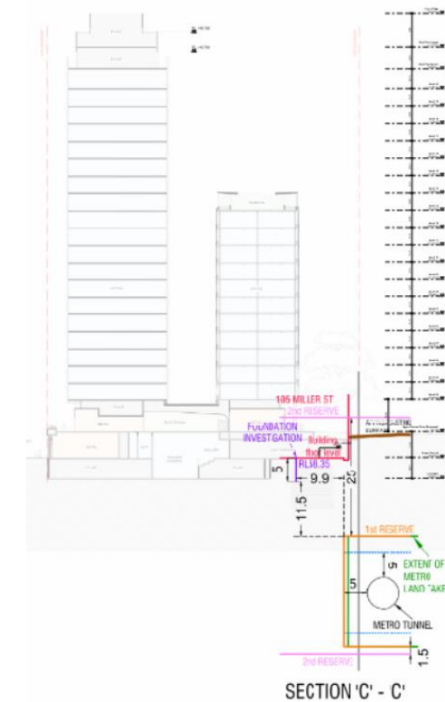
Figure 5 Impact on Metro - Section
