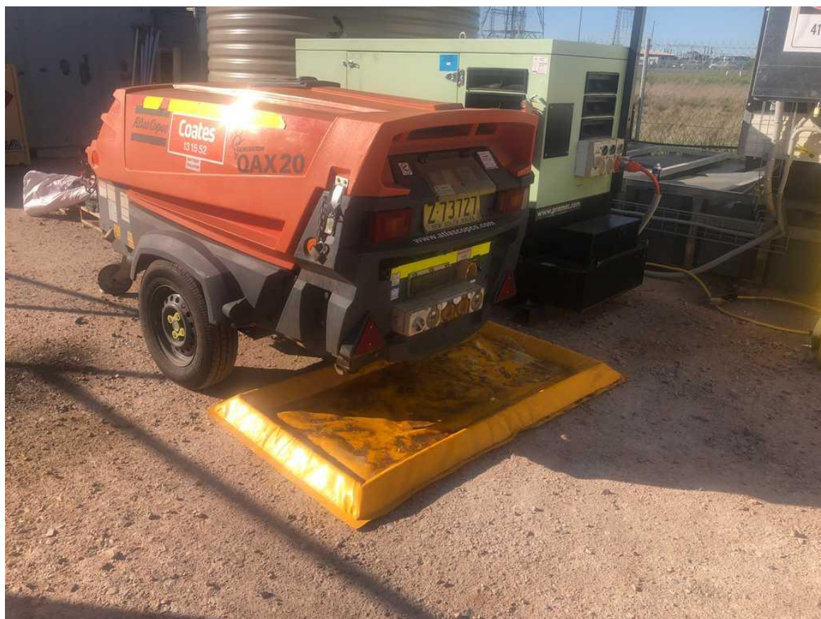
Photo 7– Spill containment measure underneath diesel generator
