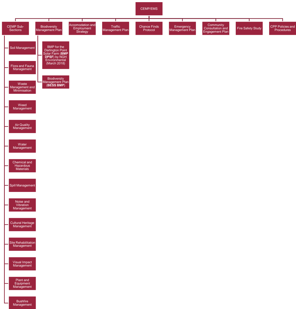
Figure 1 Structure of the CEMP/EMS for the Project
