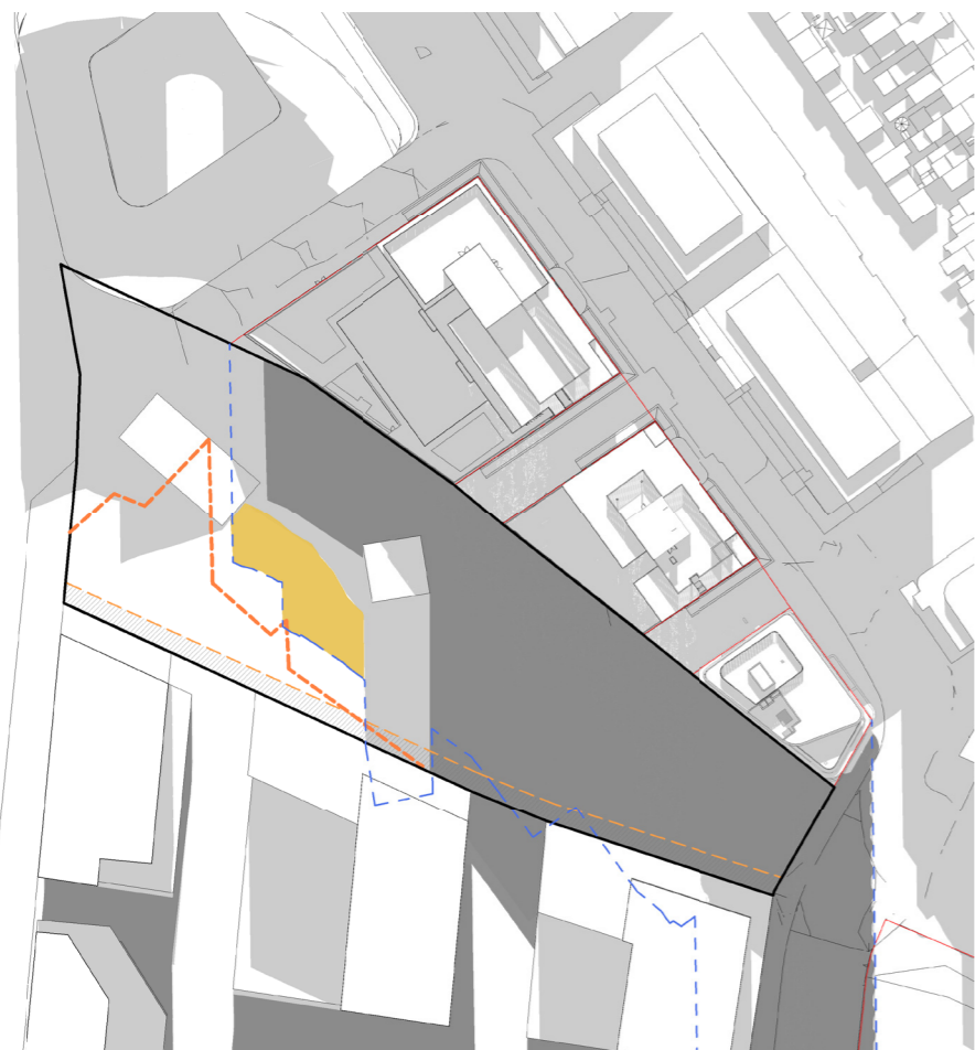
At 12pm on June 21 st an additional 430 m 2 of the plaza receives direct sunlight compared to the Planning Envelope and DCP controls.
