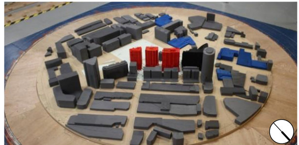
Image 2b: Wind Tunnel Study Model - Proposed Configuration
