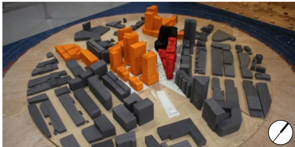
Image 2c: Wind Tunnel Study Model - Future Configuration
