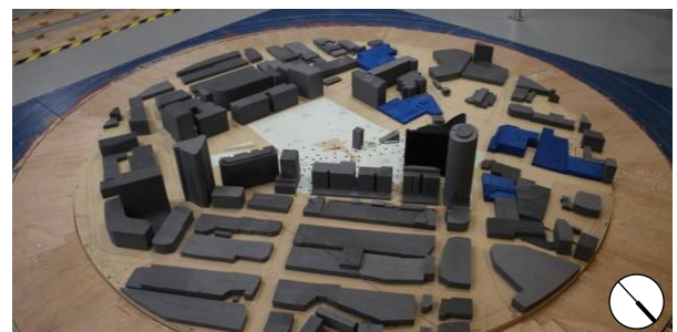
Image 2a: Wind Tunnel Study Model – Existing Configuration
