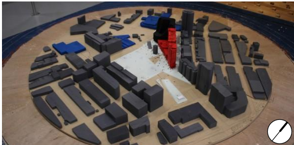
Image 2b: Wind Tunnel Study Model - Proposed Configuration
