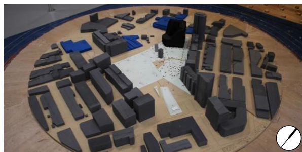
Image 2a: Wind Tunnel Study Model – Existing Configuration
