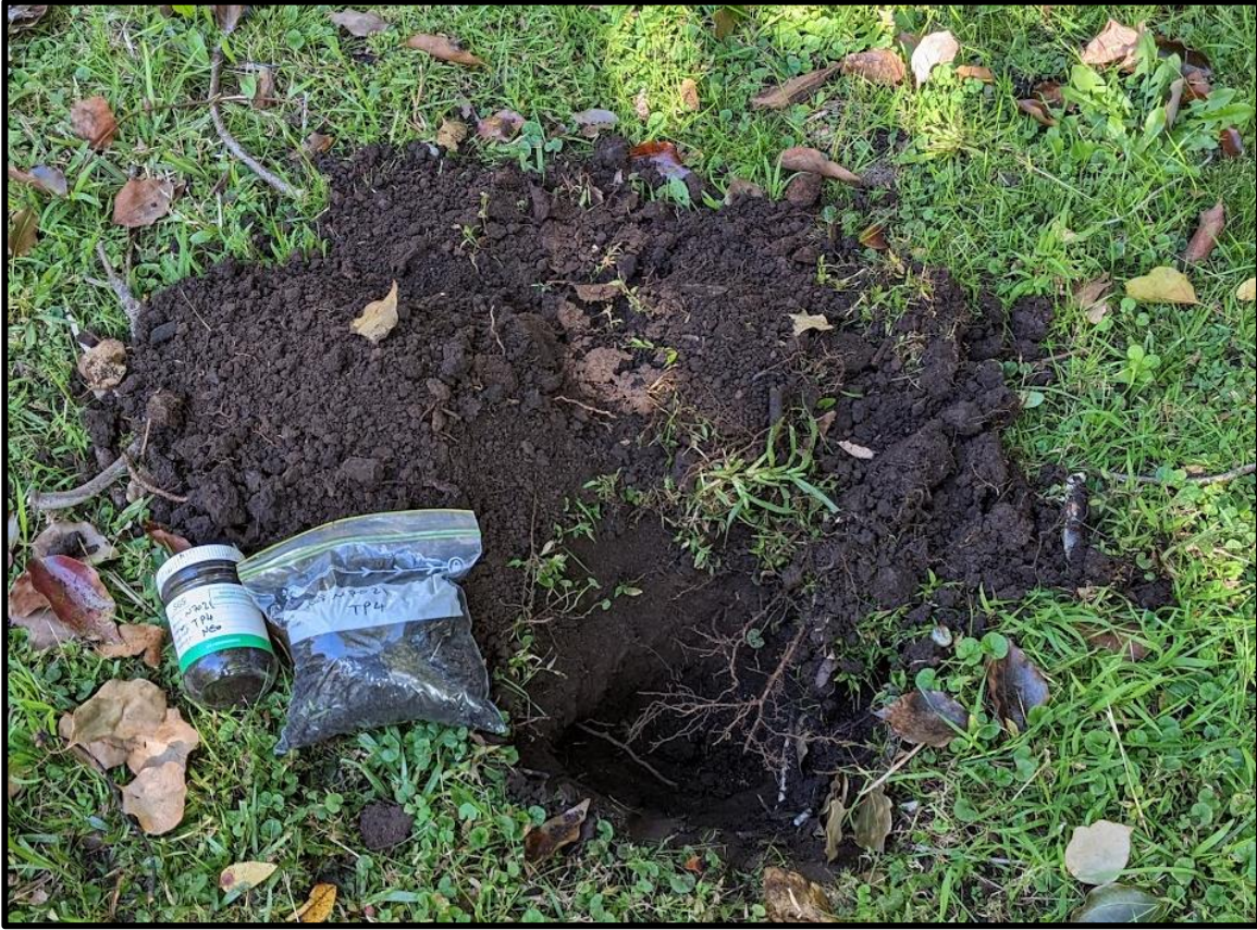
Figure 23. TP4 excavation and sampling.
