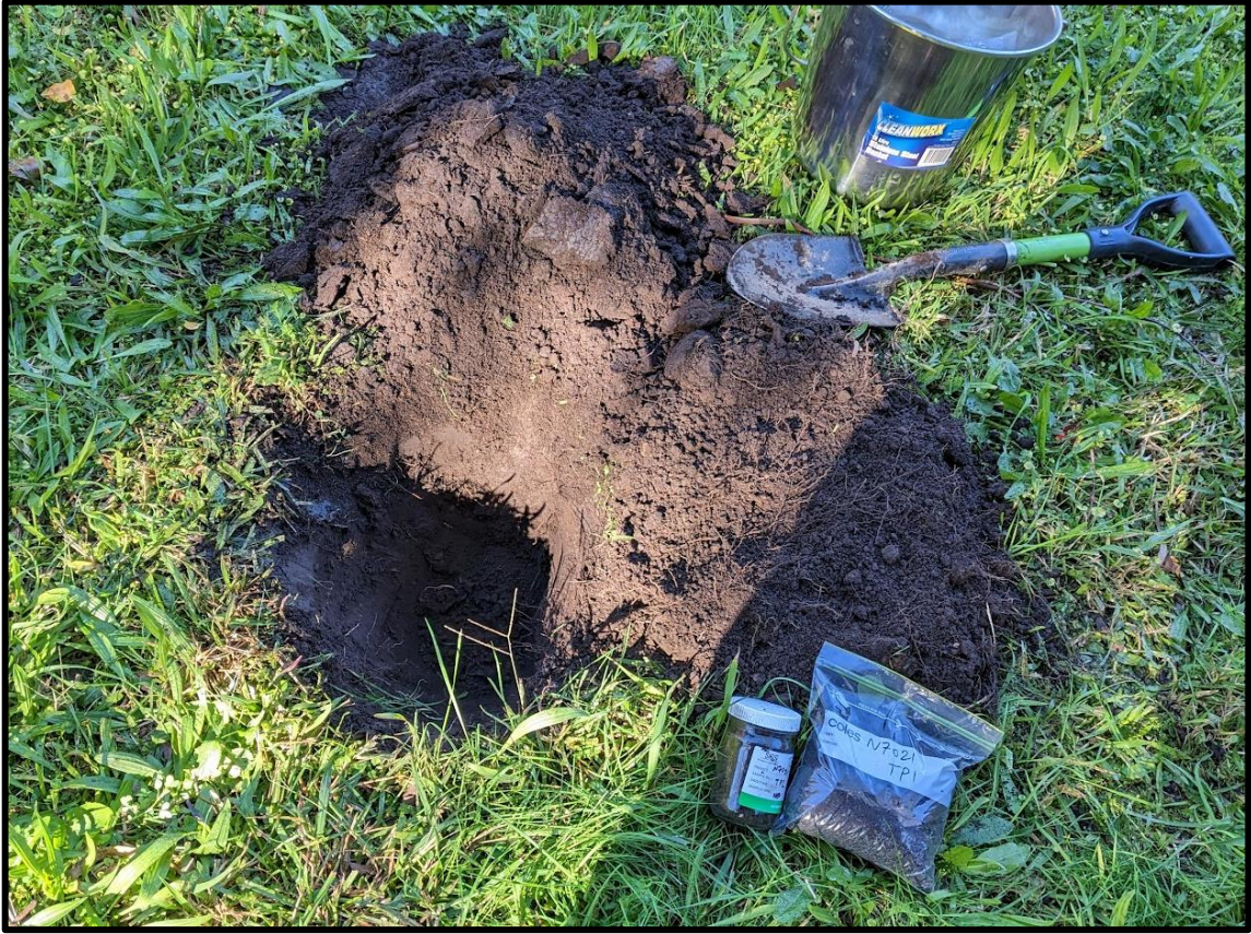
Figure 22. TP1 excavation and sampling.
