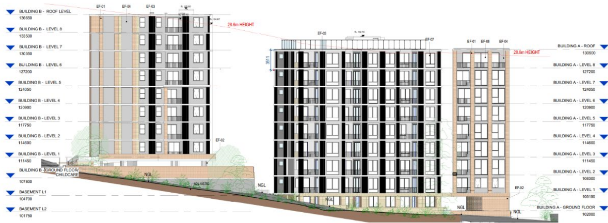
Figure 7 Proposed Western Elevation (Building B left, Building A2 centre and Building A2 right)
