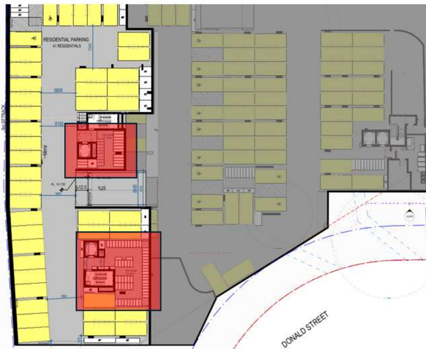
Figure 12 Bike Parking in Upper Basement Level
