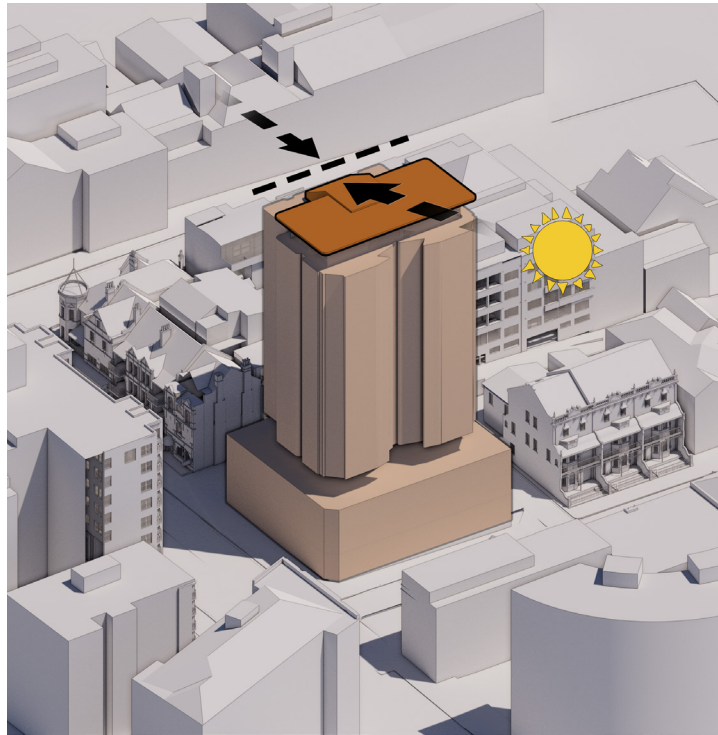
6. Locate a recessive glazed pavilion above the indicative allowable envelope where it has minimal visual impact and position it so that it does not contribute any significant overshadowing.
