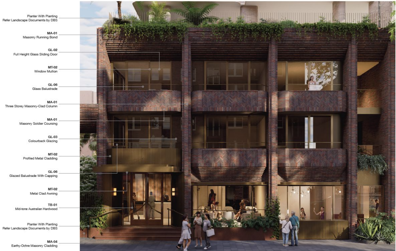
Figure 15 Podium facade materiality
