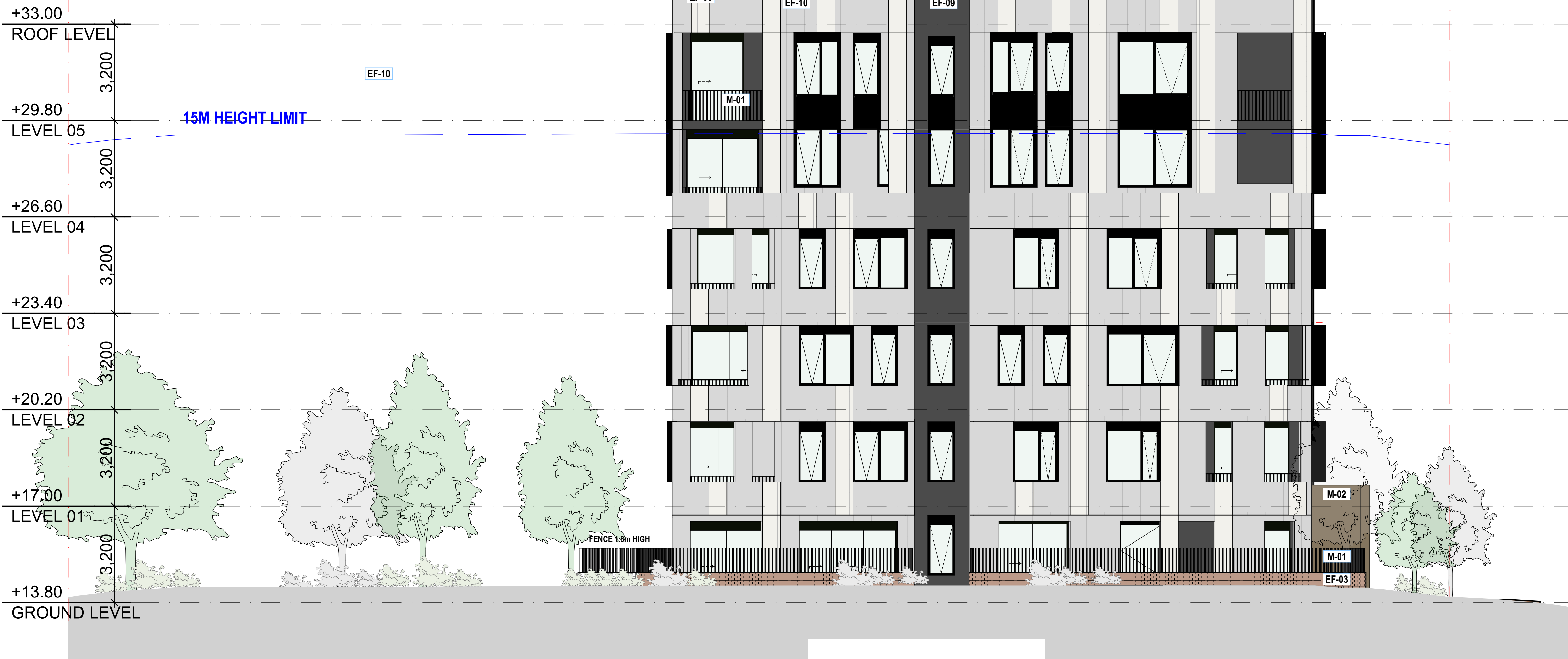
1 BUILDING 2.3 - NORTH ELEVATION 1:80
