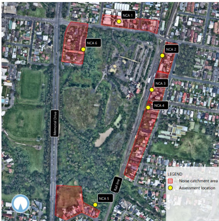
Figure 31: Residential Noise Catchment Areas and Assessment Locations
