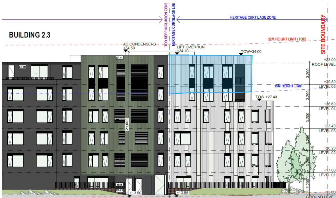
Figure 7 Exceedance of LEP Building Height Development Standard
