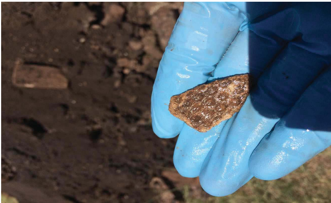
Photograph 10: Bonded ACM fragment identified within test pit. Fill building materials excavated from test pit in the background (onto black plastic material).
