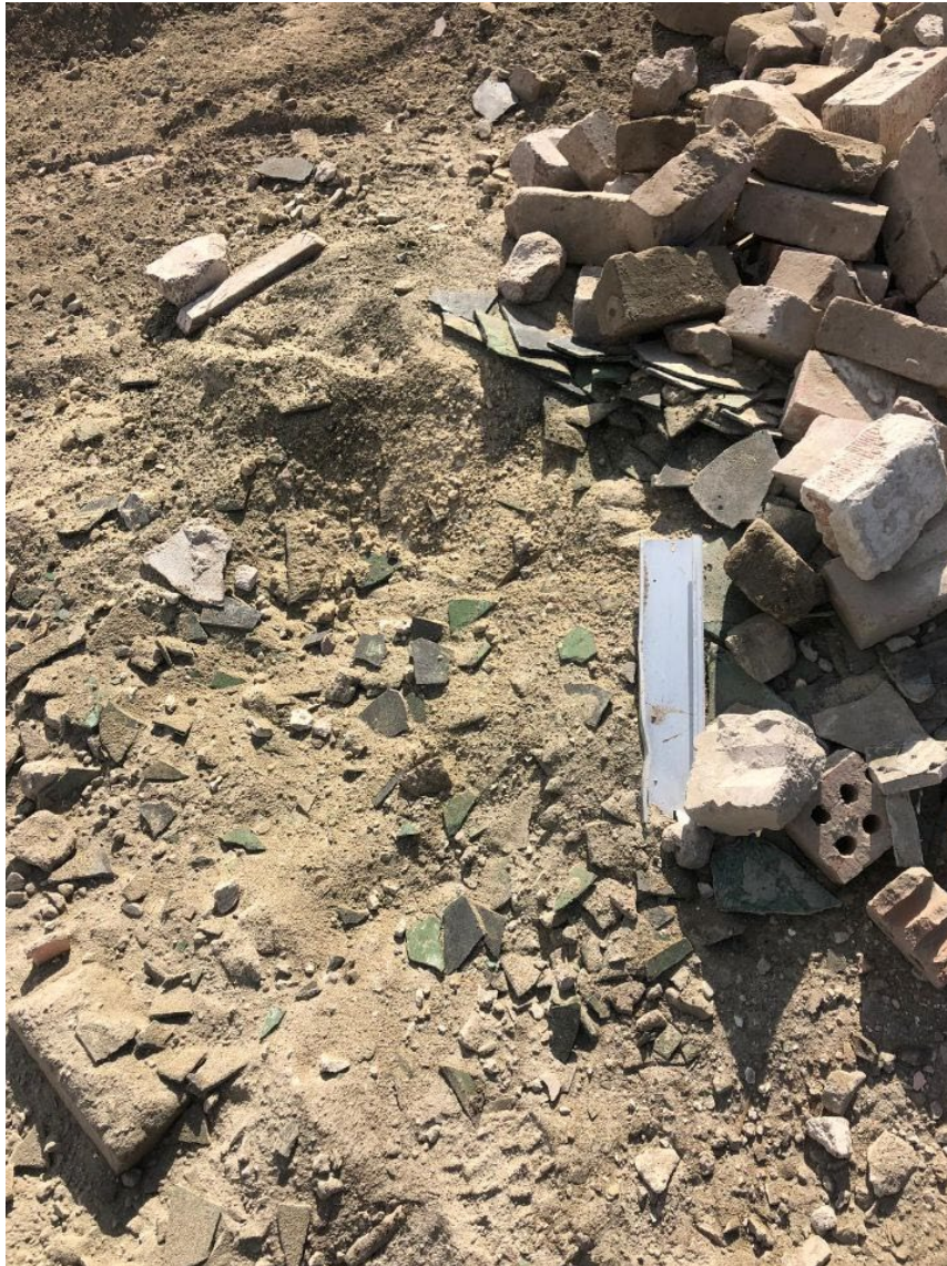
Stockpiled fill soil containing asbestos cement sheet debris in the Block A area at the Penshurst Public School, Forest Road, Penshurst NSW on 21 May 2019
