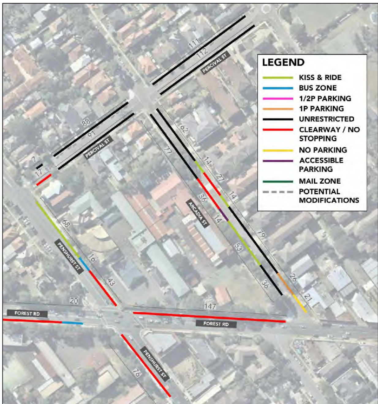
Figure 14: Existing parking controls within the vicinity of Penshurst Public School
