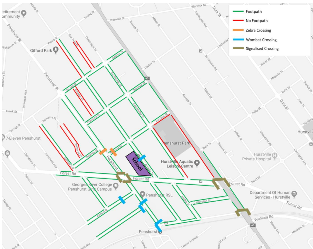
Figure 4 - Existing Footpaths and Pedestrian Crossing
