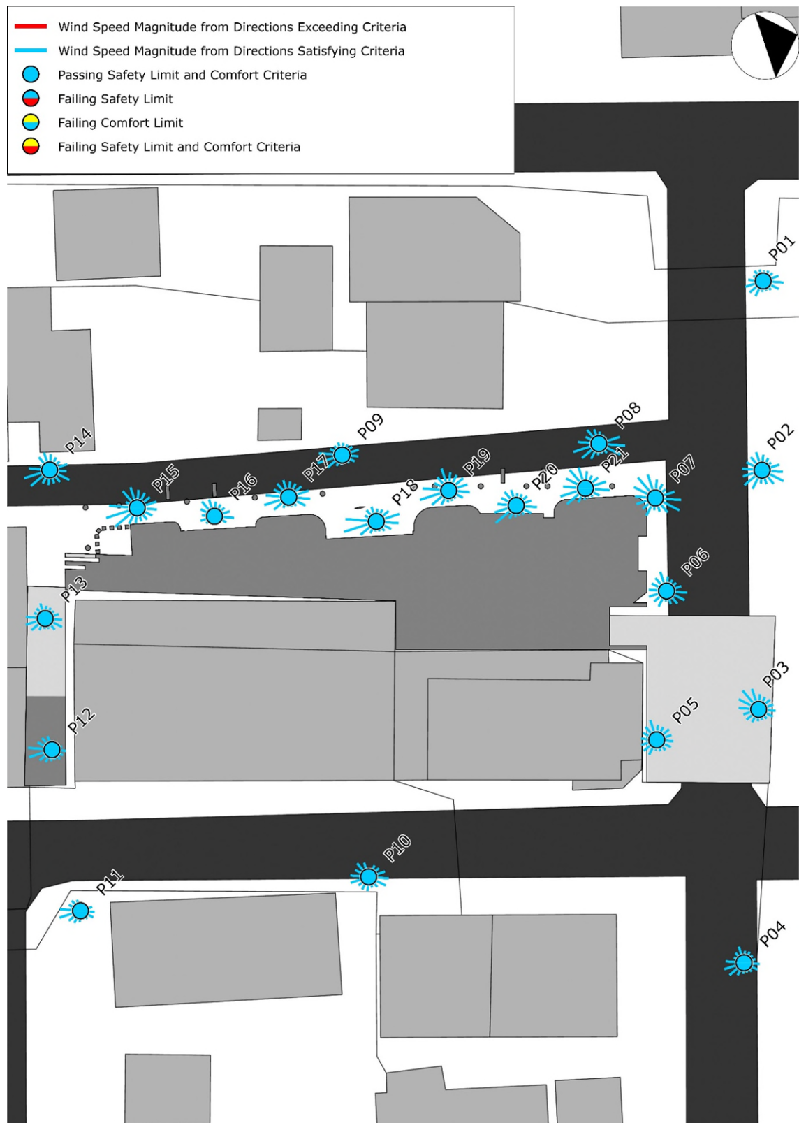
Figure 6a: Wind Tunnel Results – Ground Level Plan (results shown without treatments applied)
