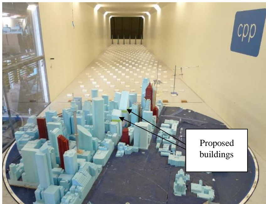
Figure 7: Photograph of the Martin Place Over Station development model in the CPP wind tunnel viewed from the south
