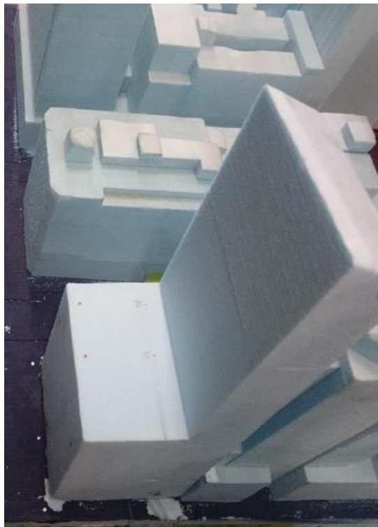
Figure 17: Wind tunnel model of the south tower with a setback of 25 m on the north façade, viewed from the west – Configuration D
