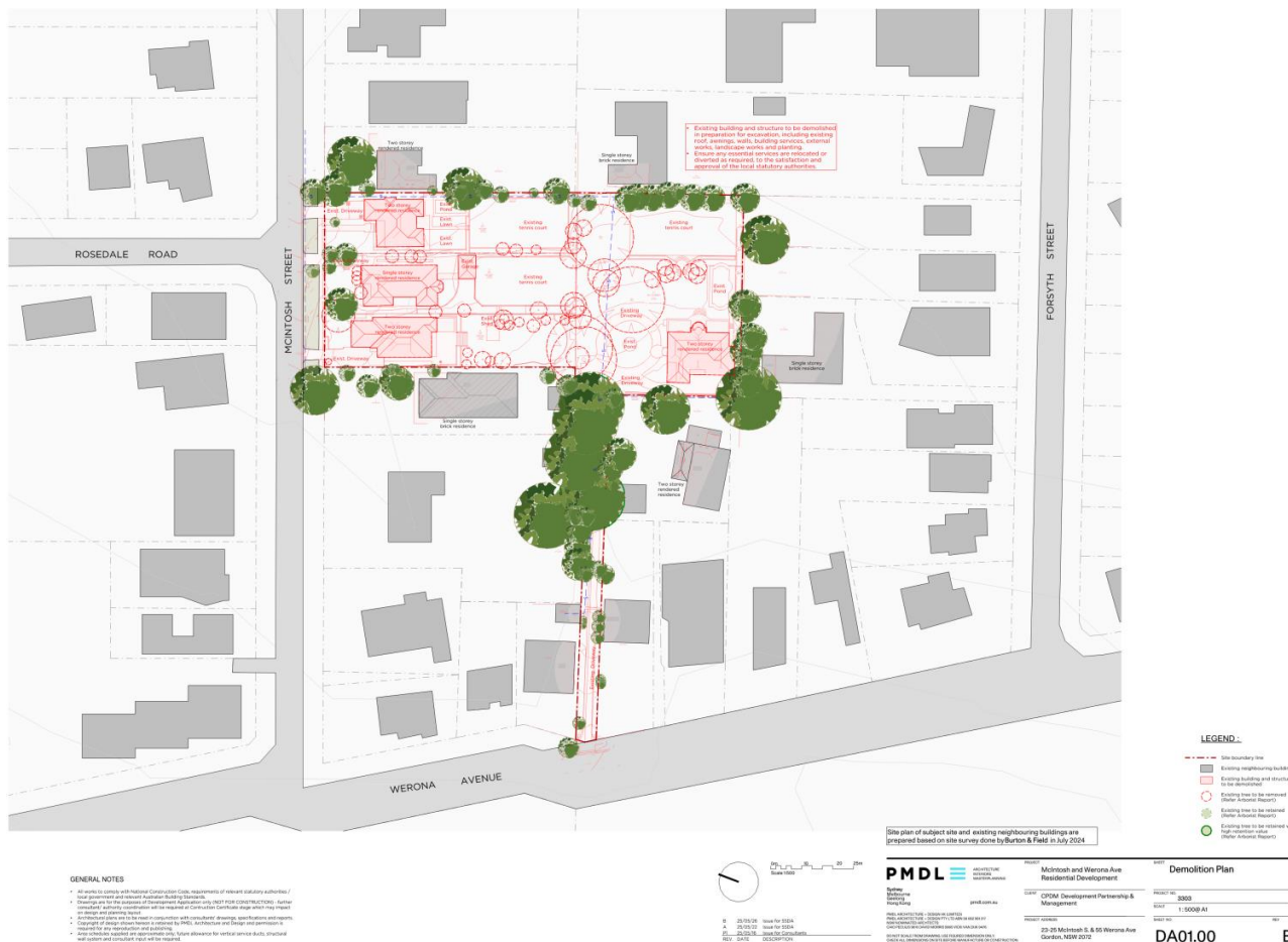
Figure 33 Demolition plan (Source: PMDL Architects)
