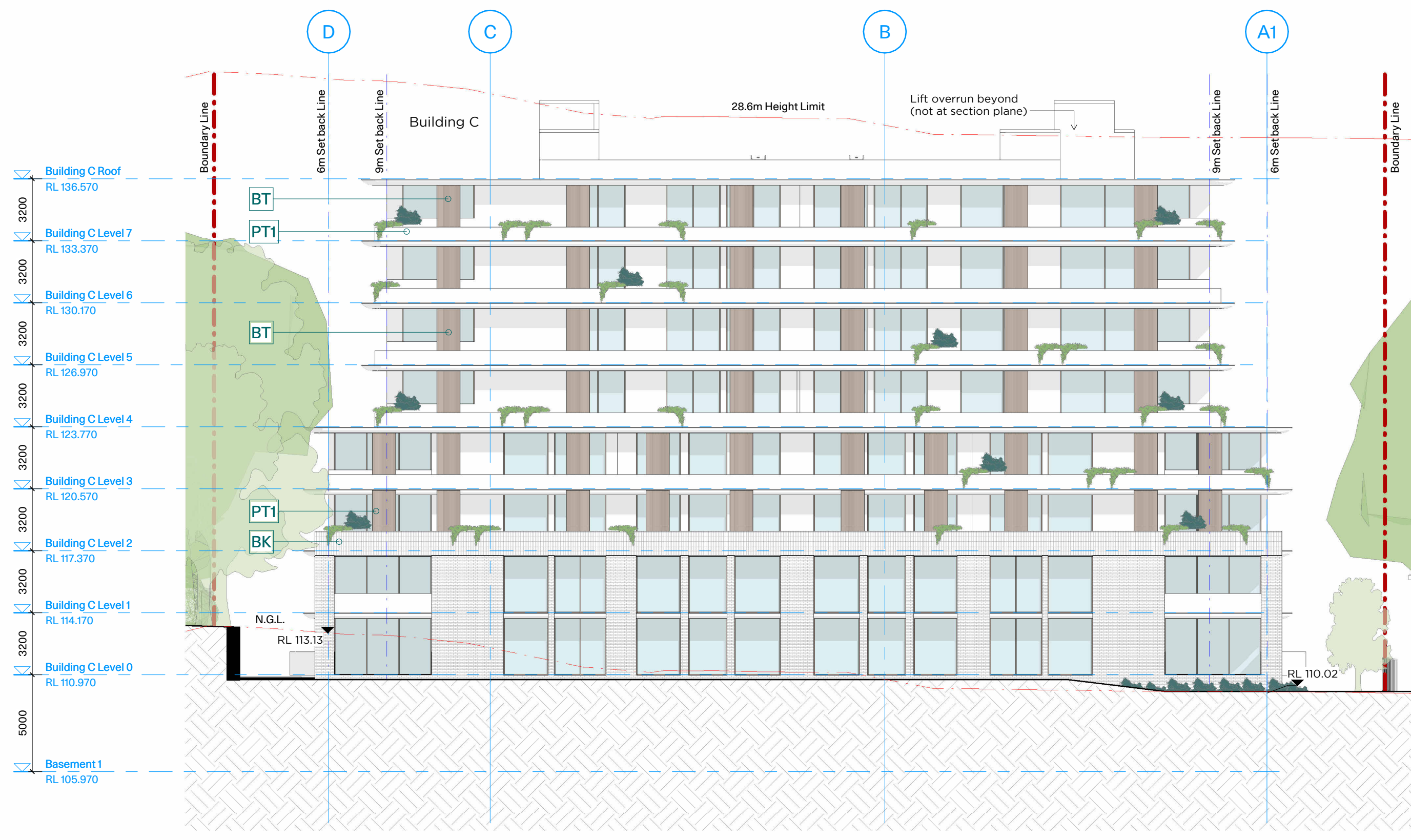
2 Building C South Elevation 1:200
