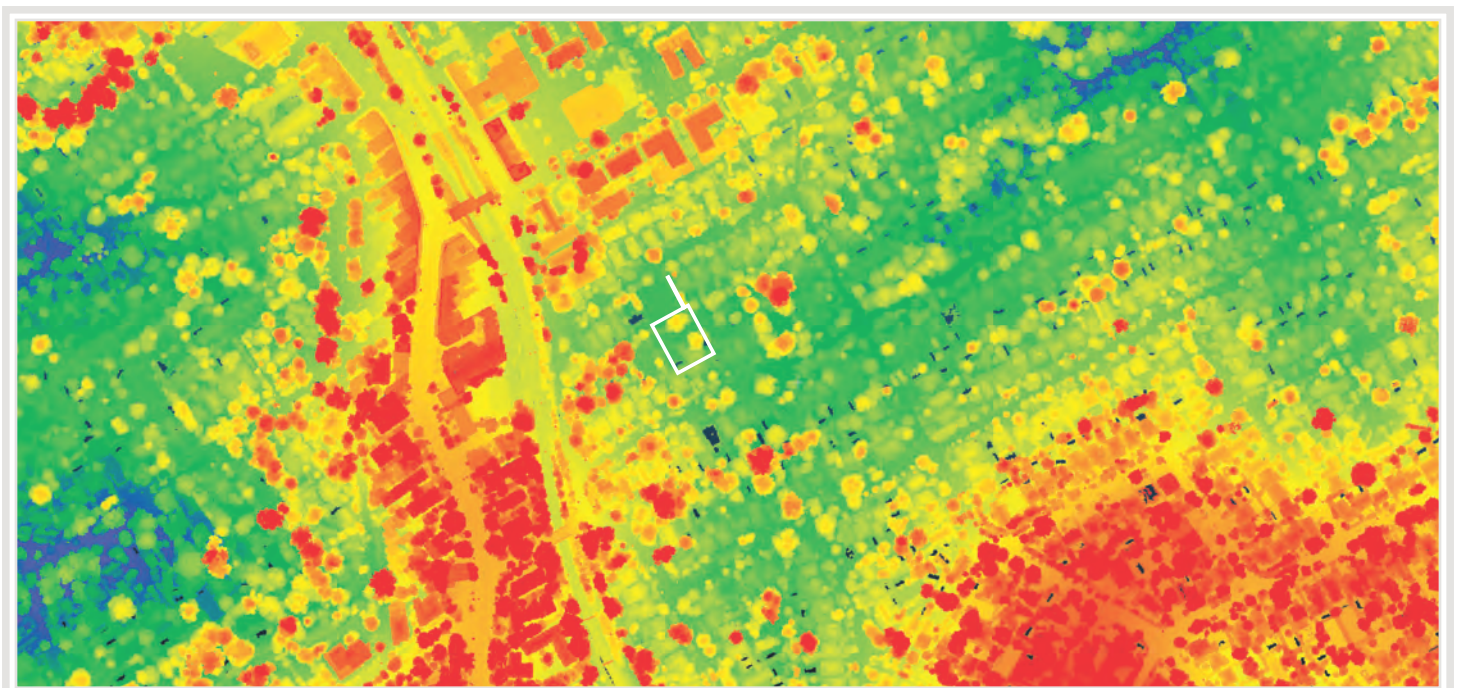
Figure 8: Lidar Point cloud including trees and buildings with gradient ramp to show topography, proposed site in white outline.
