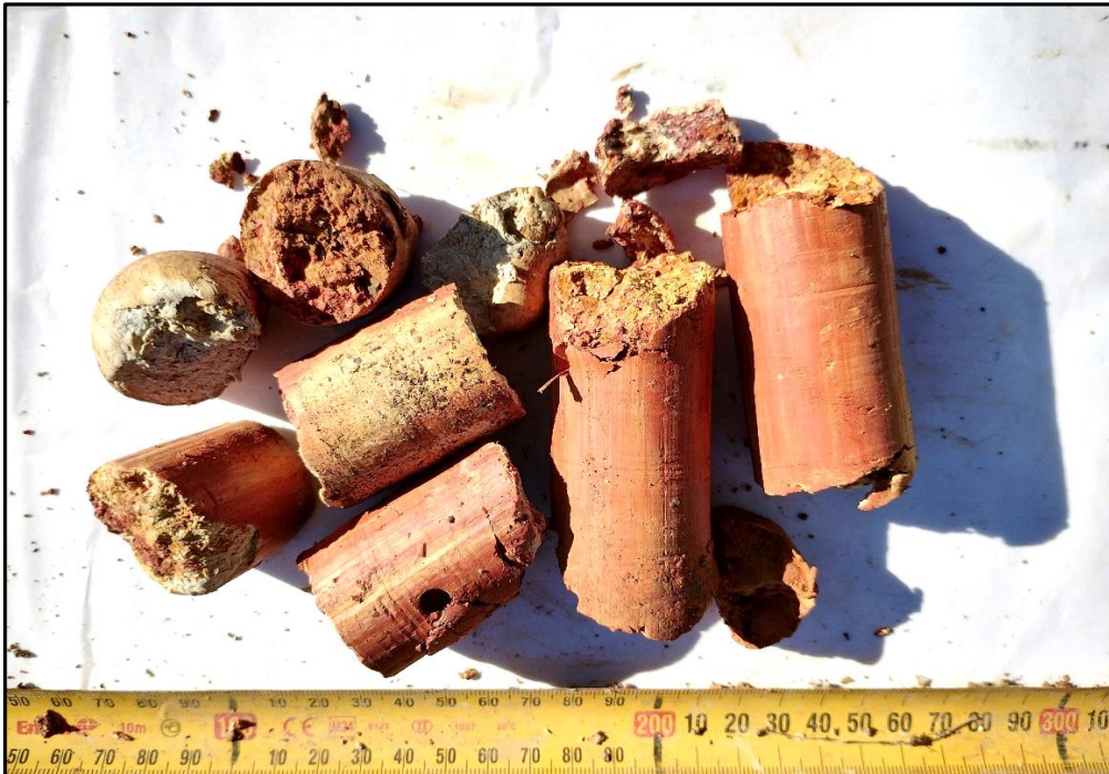
Photo 6: Bore 101 SPT Sample 1 m - 1.45 m
