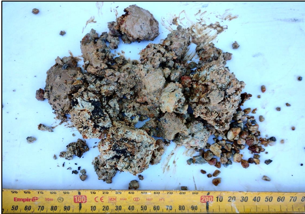
Photo 26: Bore 108 SPT Sample 11.5 m
