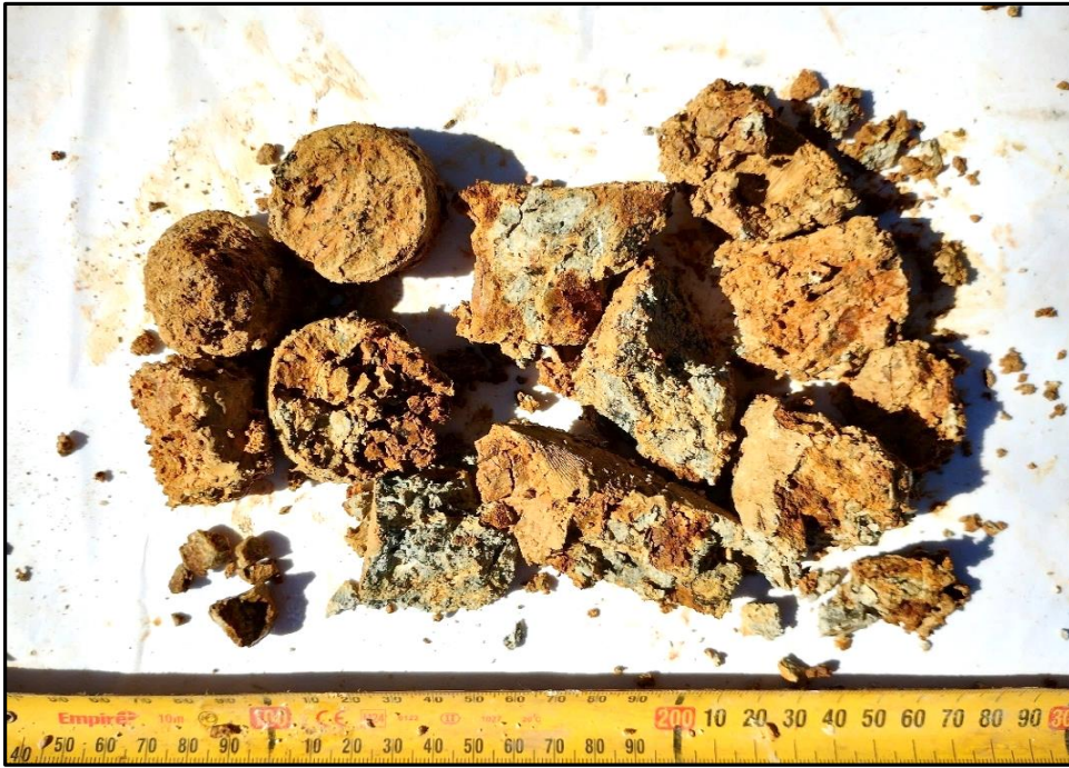
Photo 11: Bore 101 SPT Sample 8.5 m - 8.95 m
