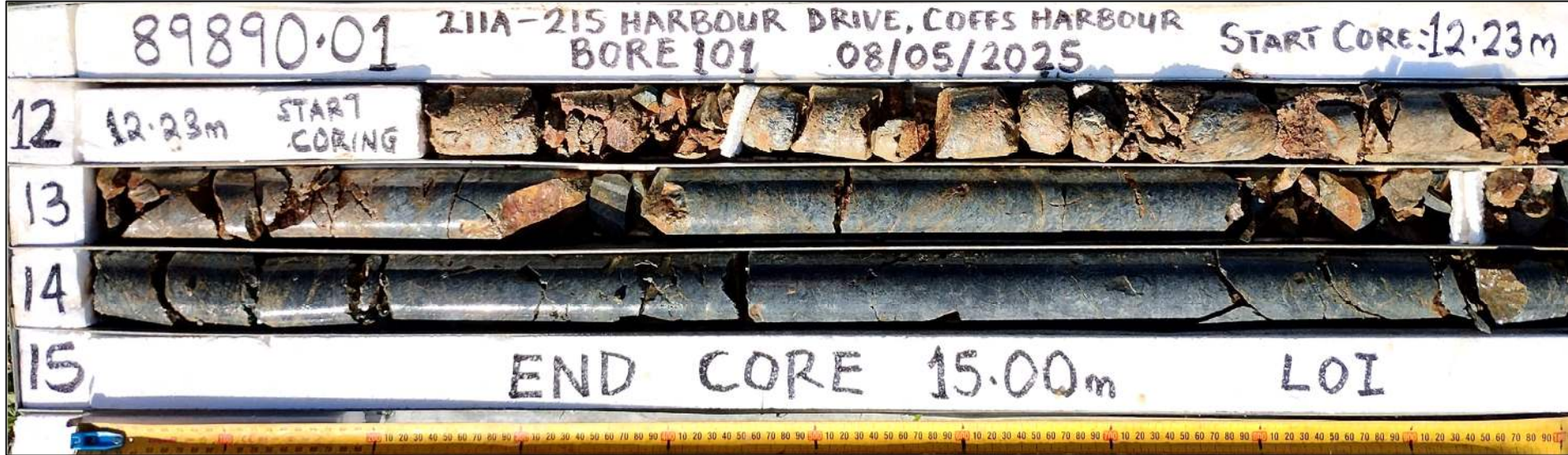
Photo 1: Bore 101 core 12.23 m to 15.00 m
