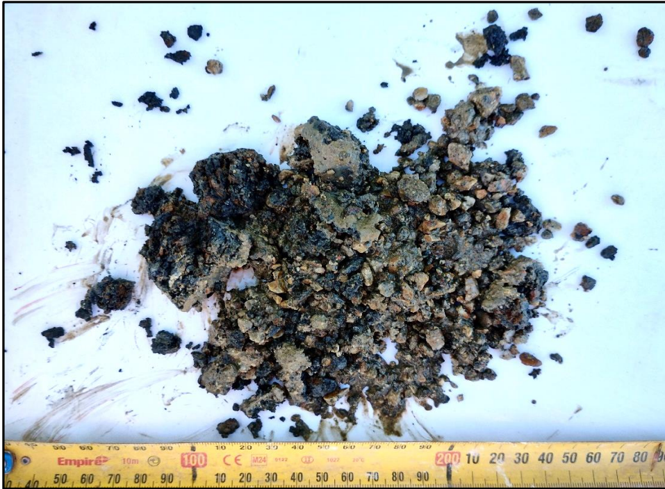
Photo 28: Bore 108 SPT Sample 13 m - 13.45 m
