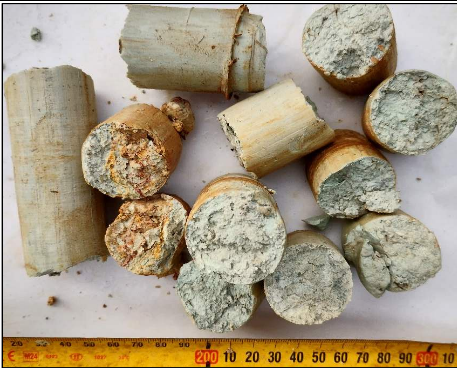
Photo 34: Bore 109 SPT Sample 4 m - 4.45 m
