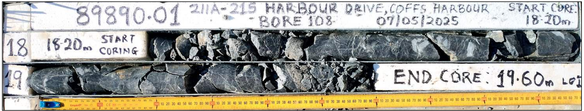
Photo 2: Bore 108 core 18.20 m to 19.60 m
