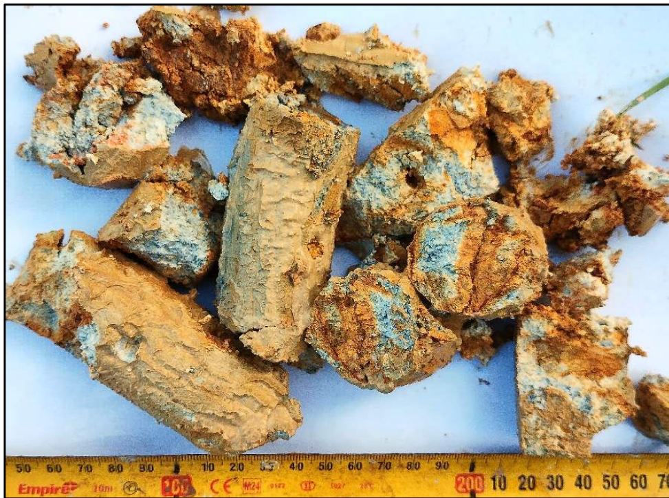
Photo 37: Bore 109 SPT Sample 8.2 m - 8.65 m
