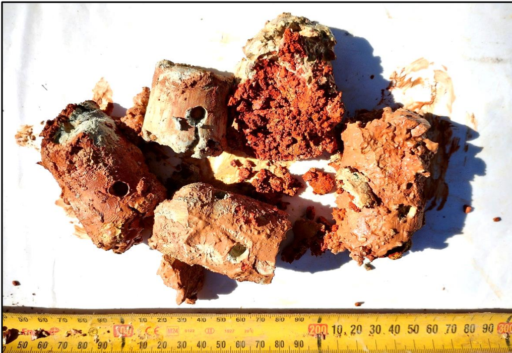
Photo 8: Bore 101 SPT Sample 4 m - 4.45 m
