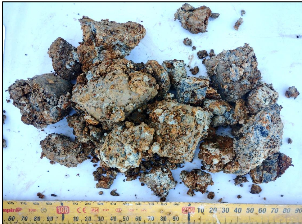
Photo 25: Bore 108 SPT Sample 10 m - 10.45 m
