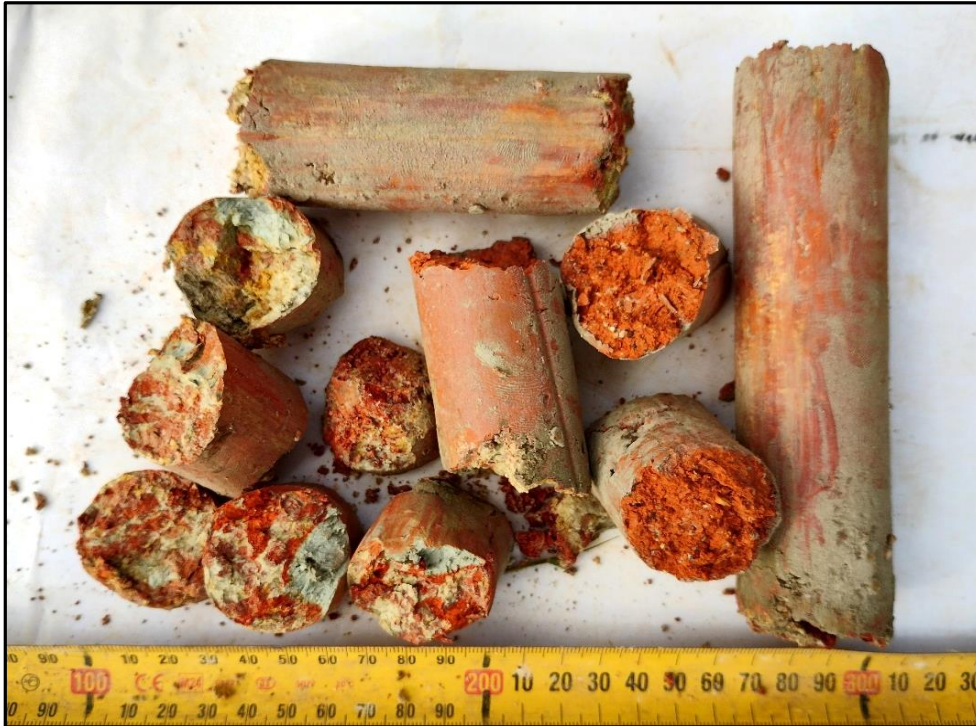
Photo 20: Bore 108 SPT Sample 2.5 m - 2.95 m
