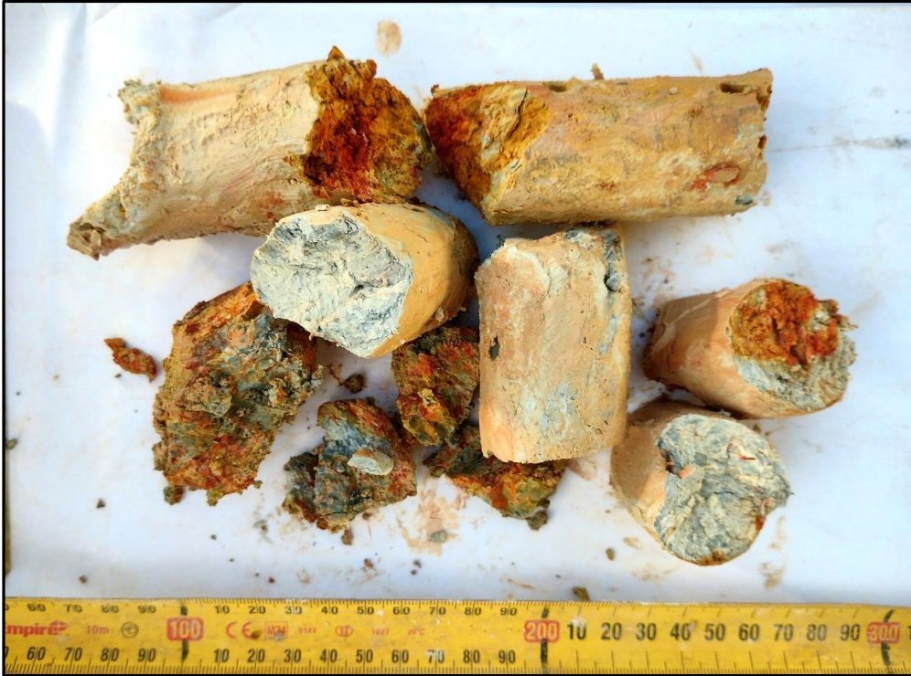
Photo 22: Bore 108 SPT Sample 5.5 m - 5.95 m
