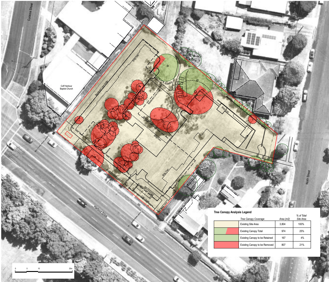
Figure 2.13 – Overall site plan showing the site and its existing urban canopy cover and relative percentages. (Source: Arterra)
