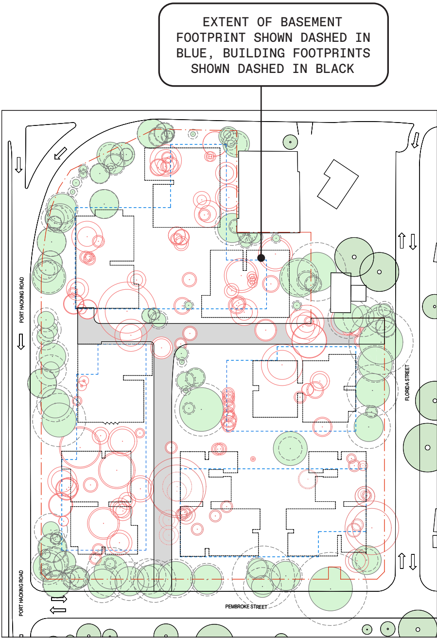
DRAWING INDICATING PROPOSED RETENTION OF ALL TREES (SHOWN GREEN) ON SITE AND PROPOSED REMOVAL OF TREES (SHOWN RED).
