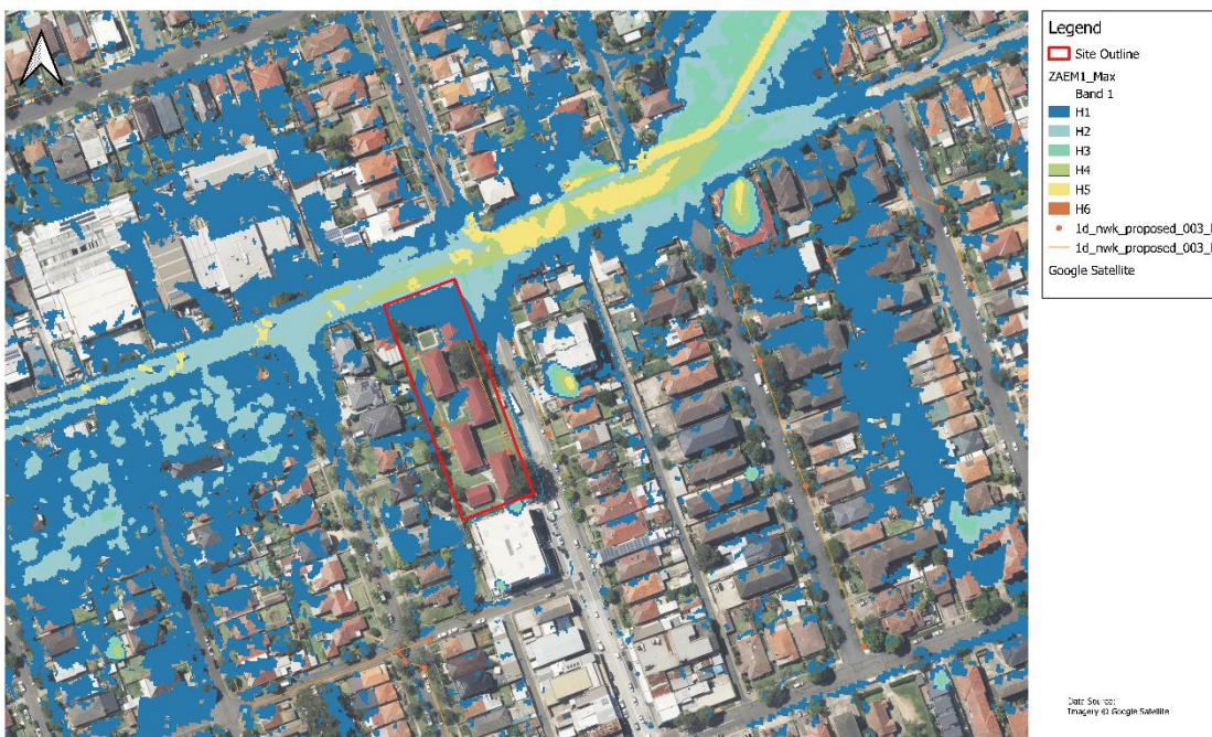
Figure 5.7: 1% AEP Post Development Flood Hazard
