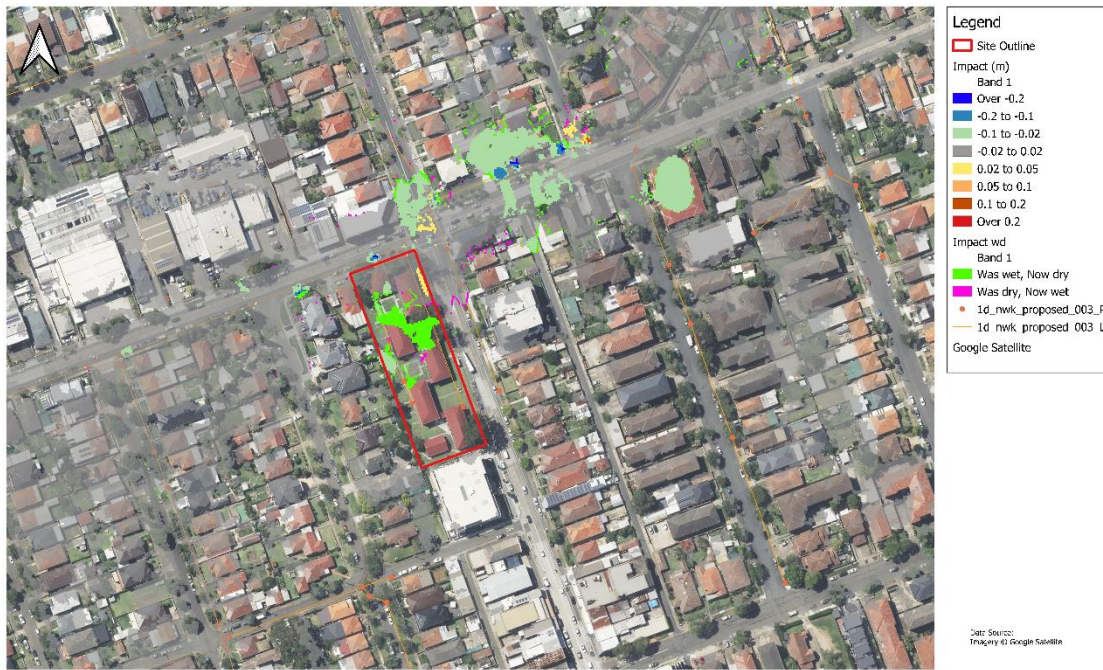
Figure 5.8: 1% AEP Flood Impact (change in water level)
