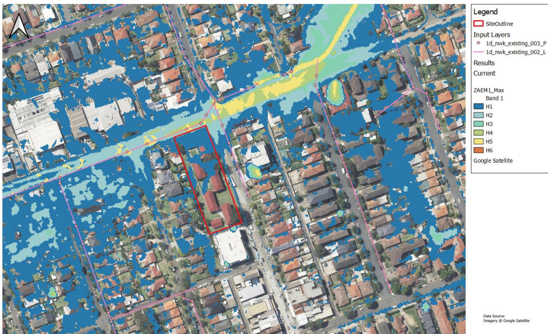
Figure 5.5: 1%AEP Existing Flood Hazard
