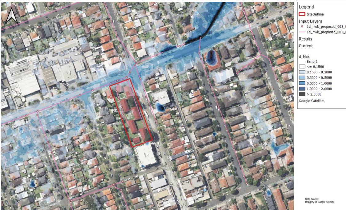
Figure 5.7: 1% AEP Post Development Flood Hazard
