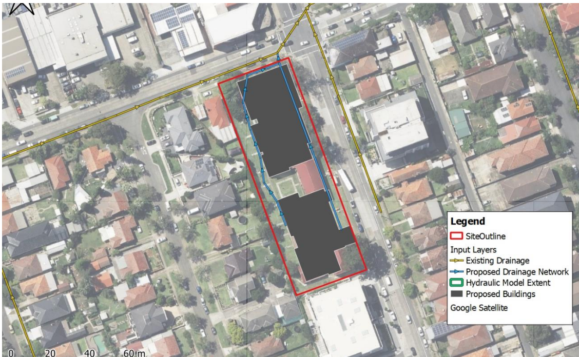
Figure 5.3: Proposed Drainage Network
