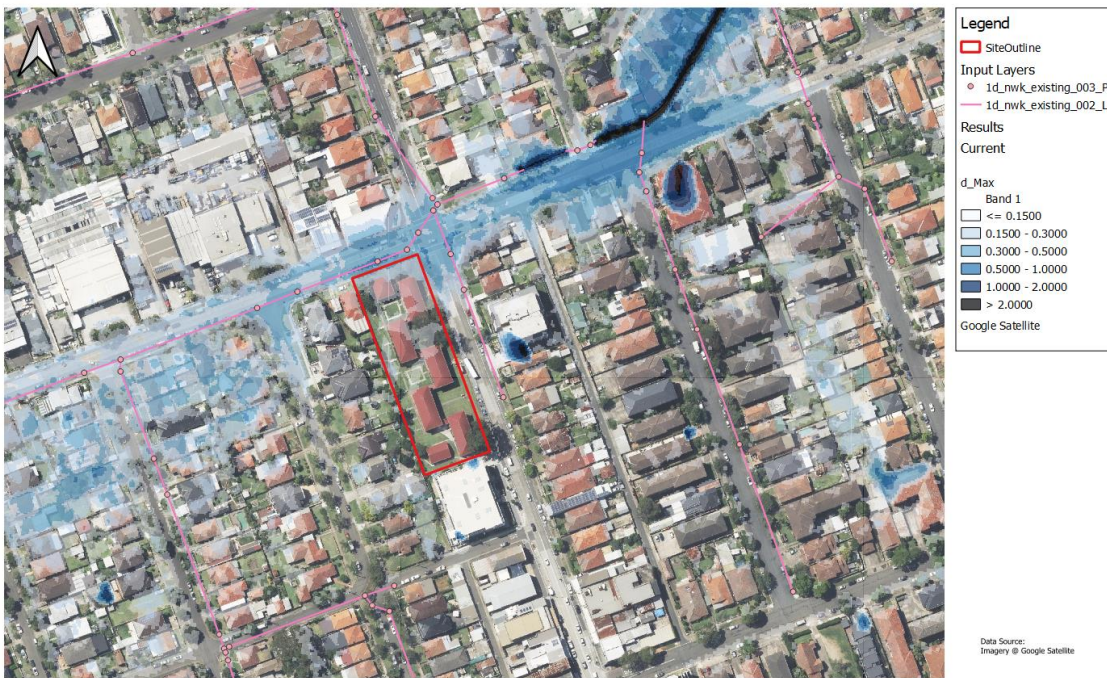
Figure 5.5: 1%AEP Existing Flood Hazard
