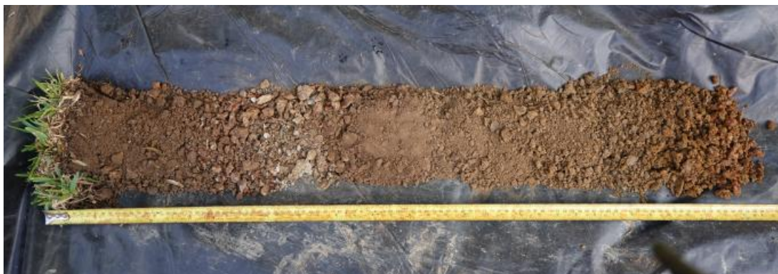
Figure 10 – Topsoil sample / profile, noting the somewhat unnatural profile with what appears to be imported topsoil material overlying a thin layer of heavy clay subsoil at 300-400mm, likely from original 1950s development of the site, before returning to a more natural existing soil profile below this disturbed surface. (Photo: Arterra 24 April 25).
