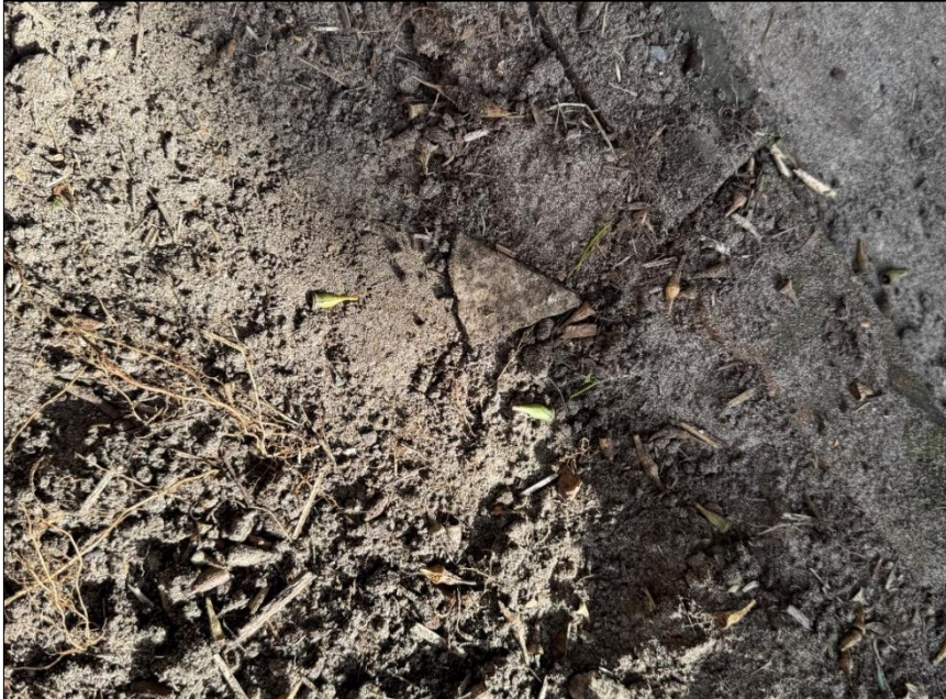
PHOTO 15. ACM FRAGMENT OBSERVED ON SURFACE NEAR BH19 (17/06/2025)
