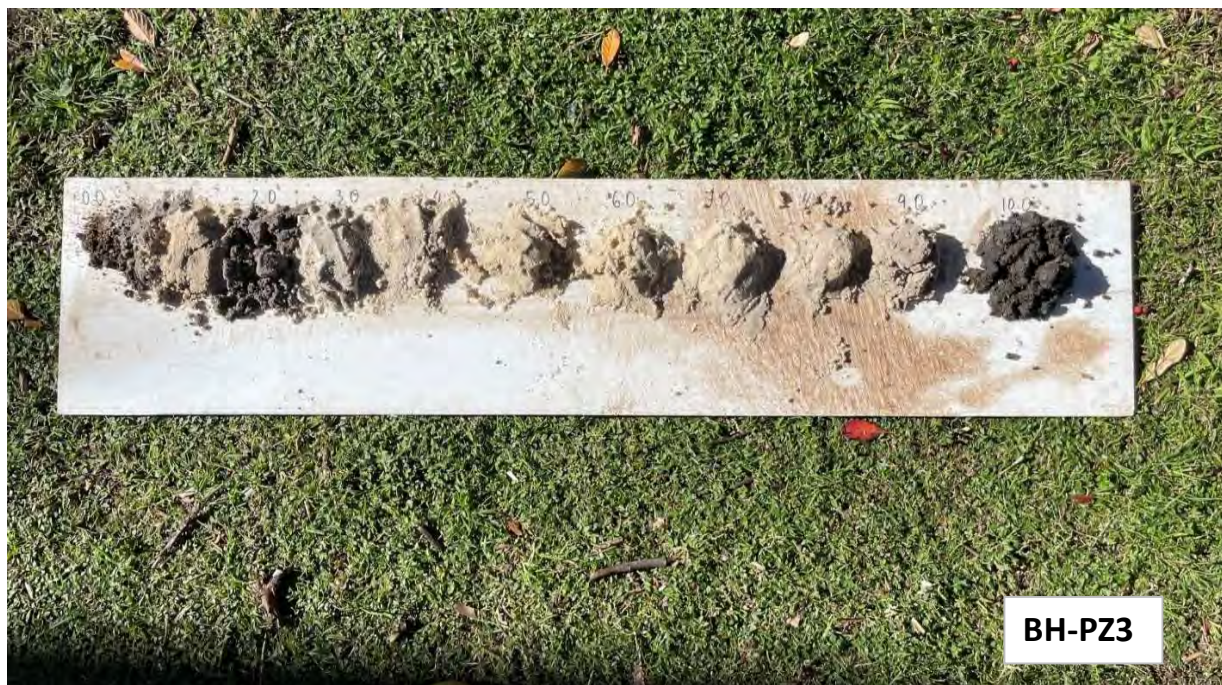
Photo 7 - Soil profile in BH-PZ3
