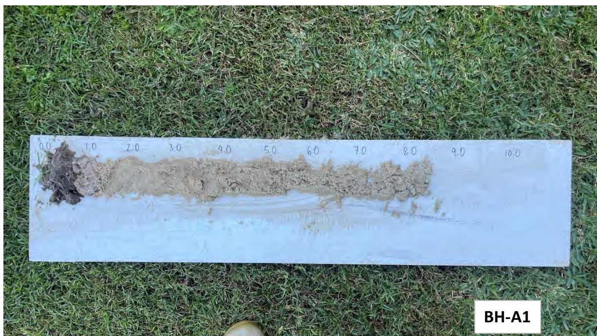
Photo 8 - Soil Profile in BH-A1
