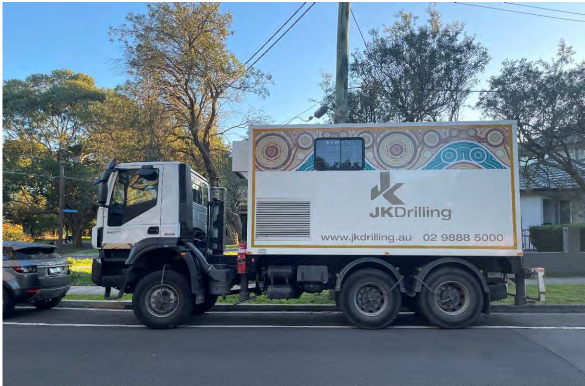
Photo 4 - JK Cone Penetration Testing Rig
