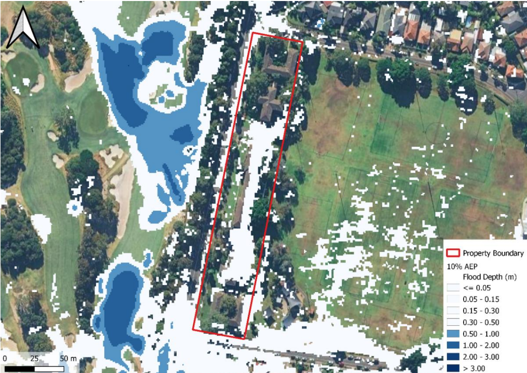
Figure 5.1: 10% AEP Flood Depth and Extent Map (Base Case)
