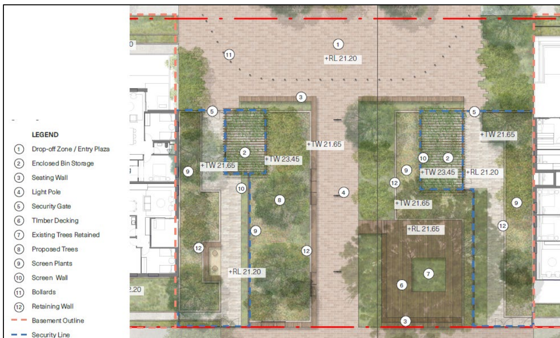
Figure 12 Setout of proposed loading area
