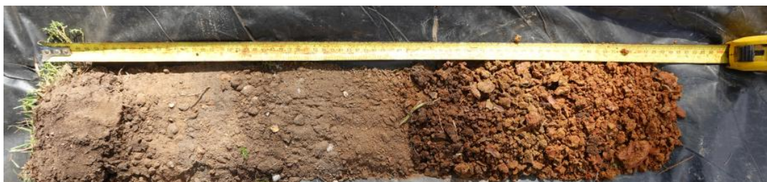
Figure 2.13 – Topsoil sample / profile, noting the somewhat unnatural profile with what appears to be imported topsoil material overlying a thin layer of heavy clay subsoil at 300-400mm, likely from original 1950s development of the site, before returning to a more natural existing soil profile below this disturbed surface. (Photos: Arterra 24 April 25).
