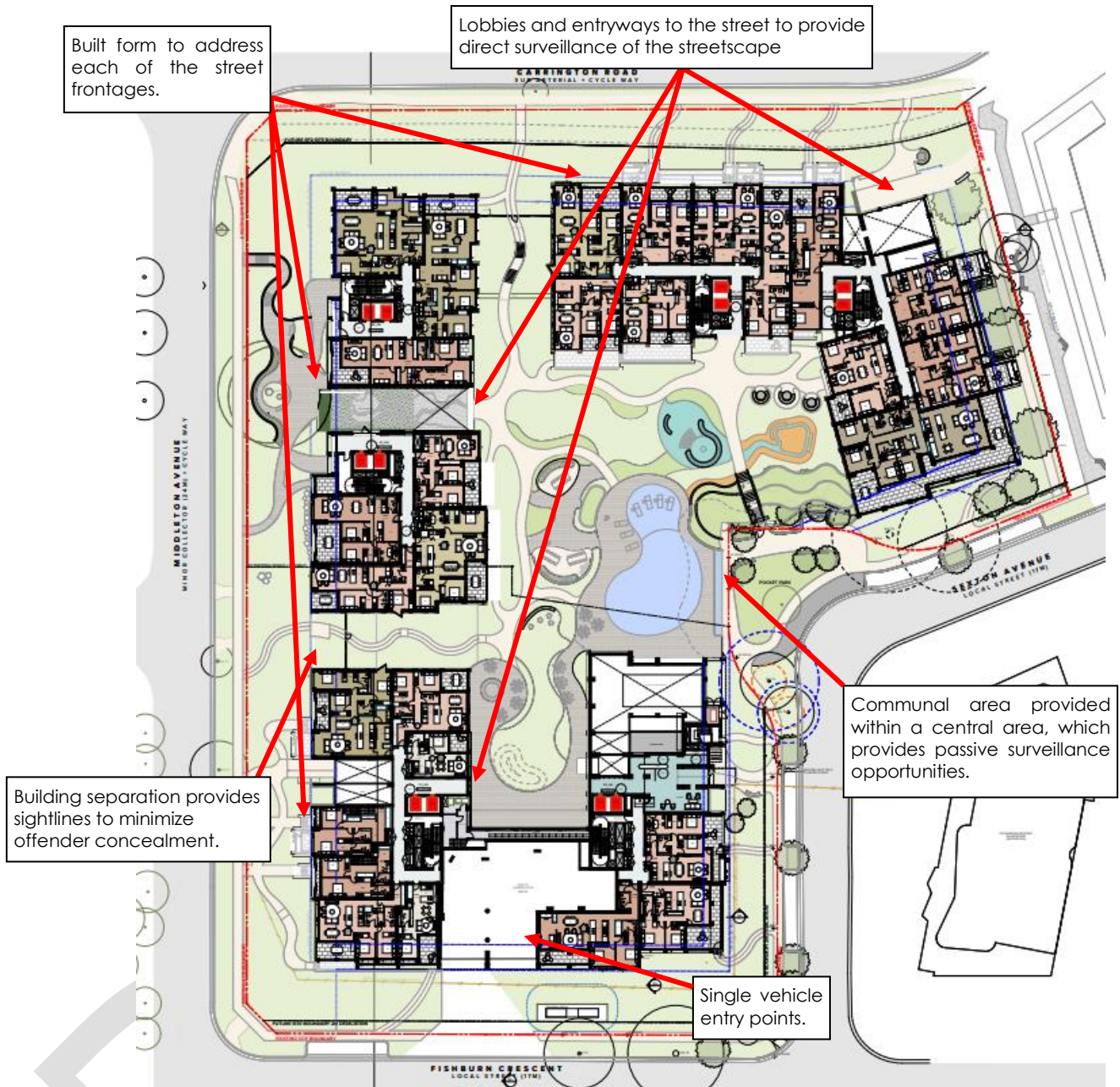
Figure 19: Extract of the ground floor plan (Turner Studio, 2025)
