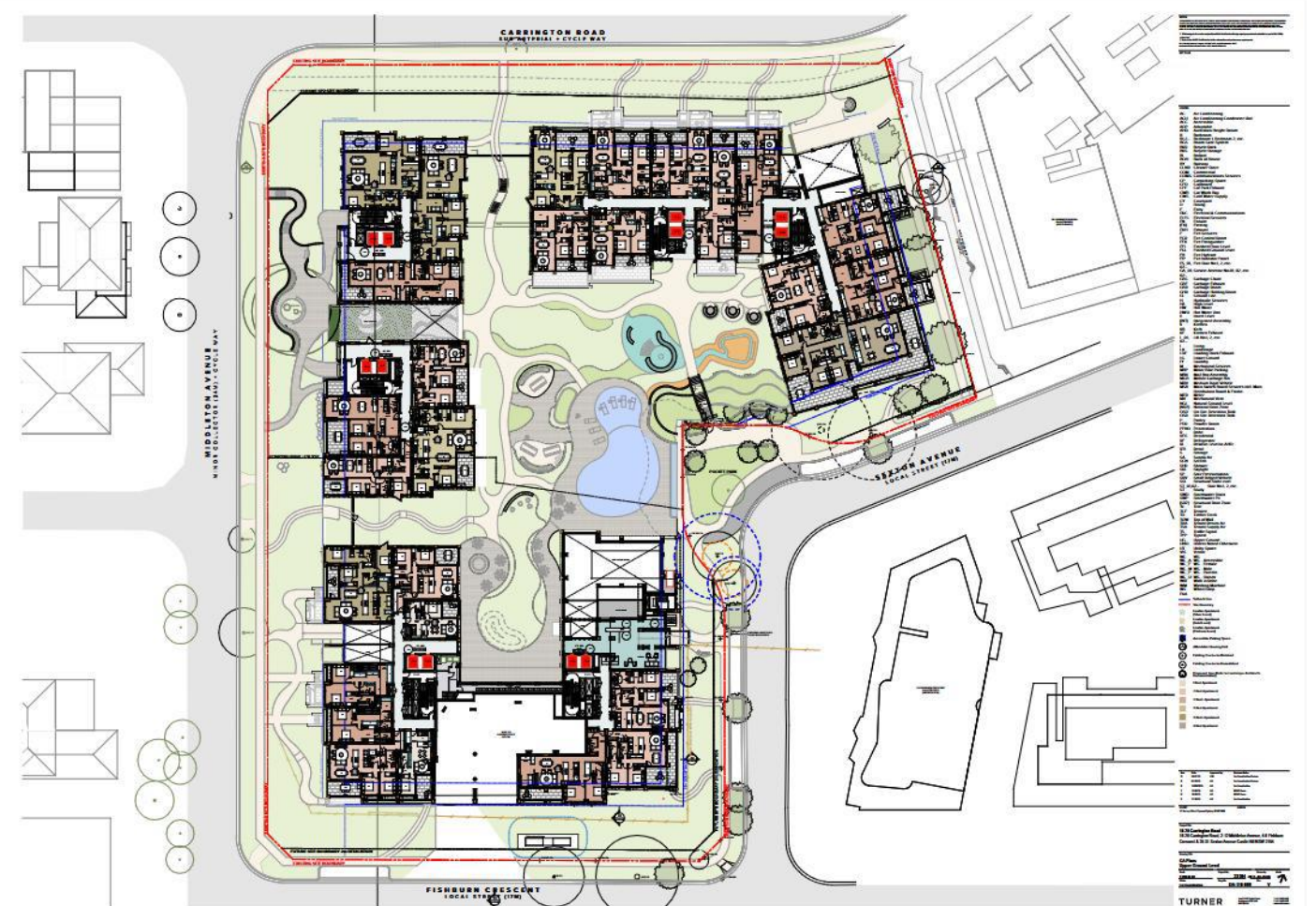
Figure 3b Upper Ground floor concept design showing the retention of existing trees along the perimeter of the study area (Turner, 2025)
