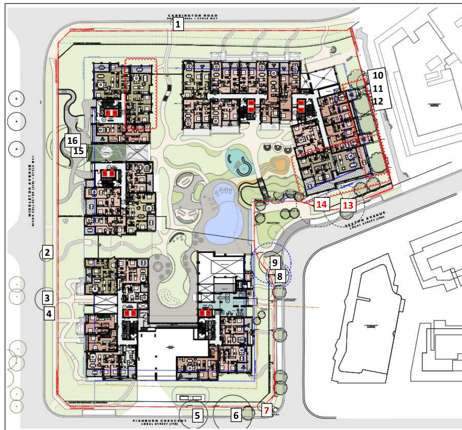
Figure 1: showing proposed design footprint & tree removal plan
