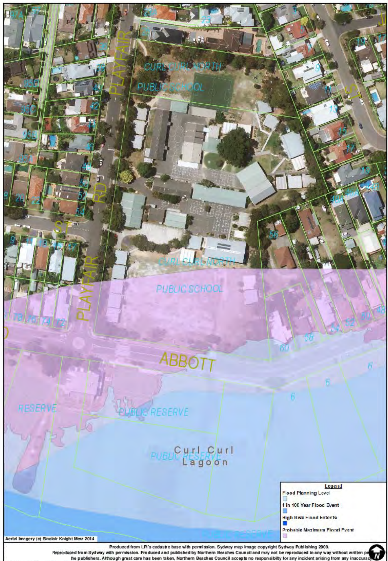
Figure 1 – Flood extents relative to the property at Curl Curl North Public School
