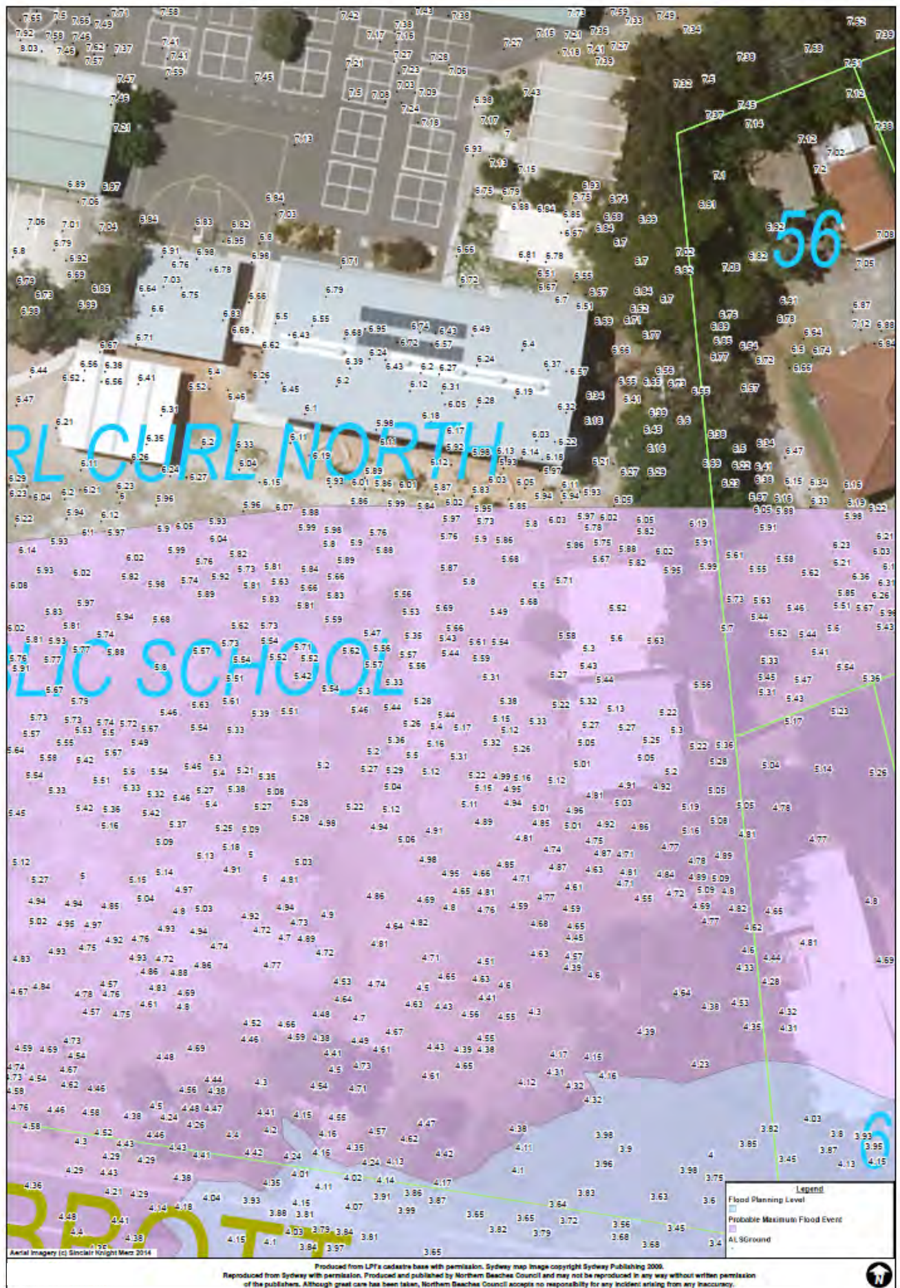
Figure 3 – Aerial Laser Survey spot heights at the property (eastern side)
