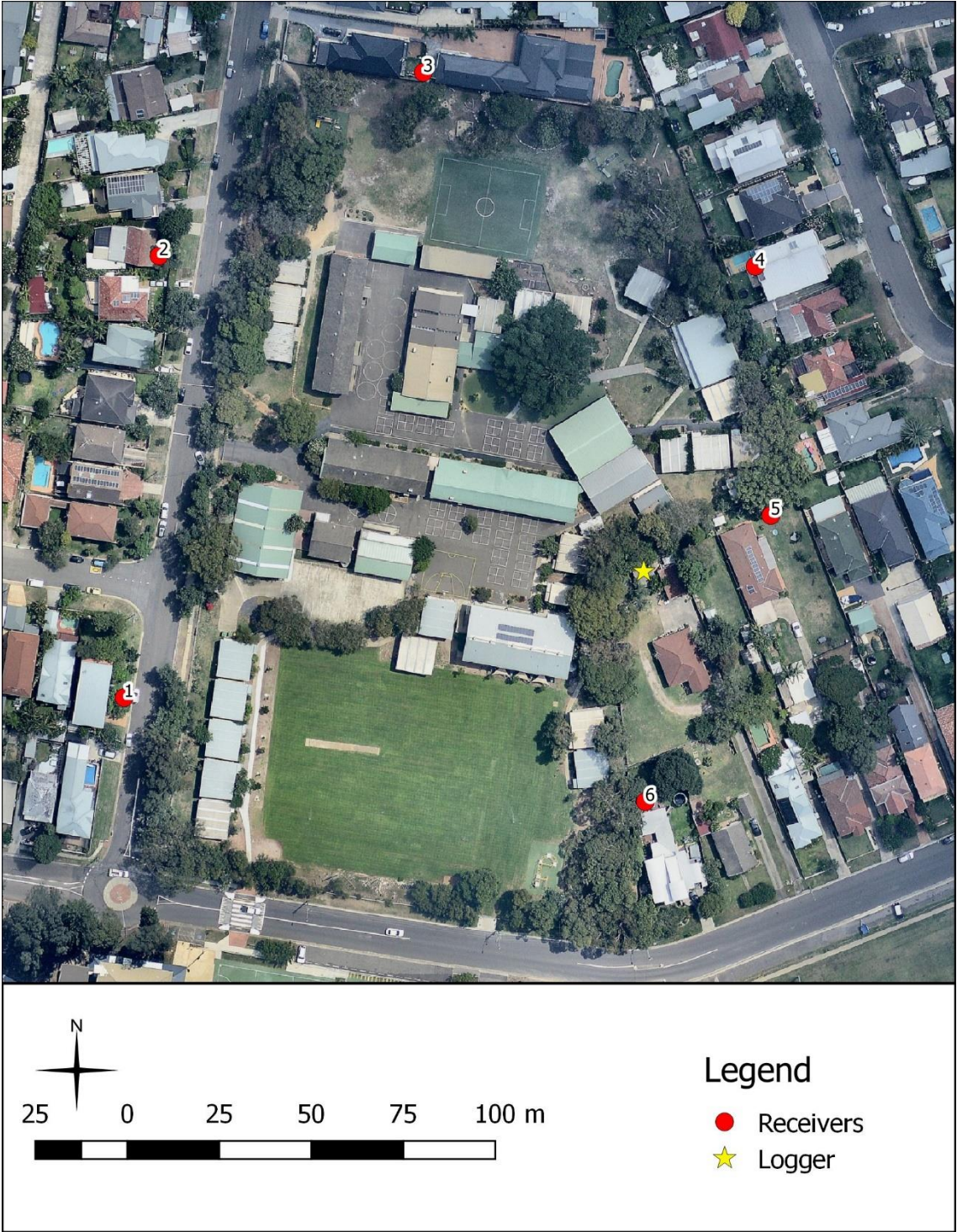
Figure 2-2 Receivers and Noise Logger
