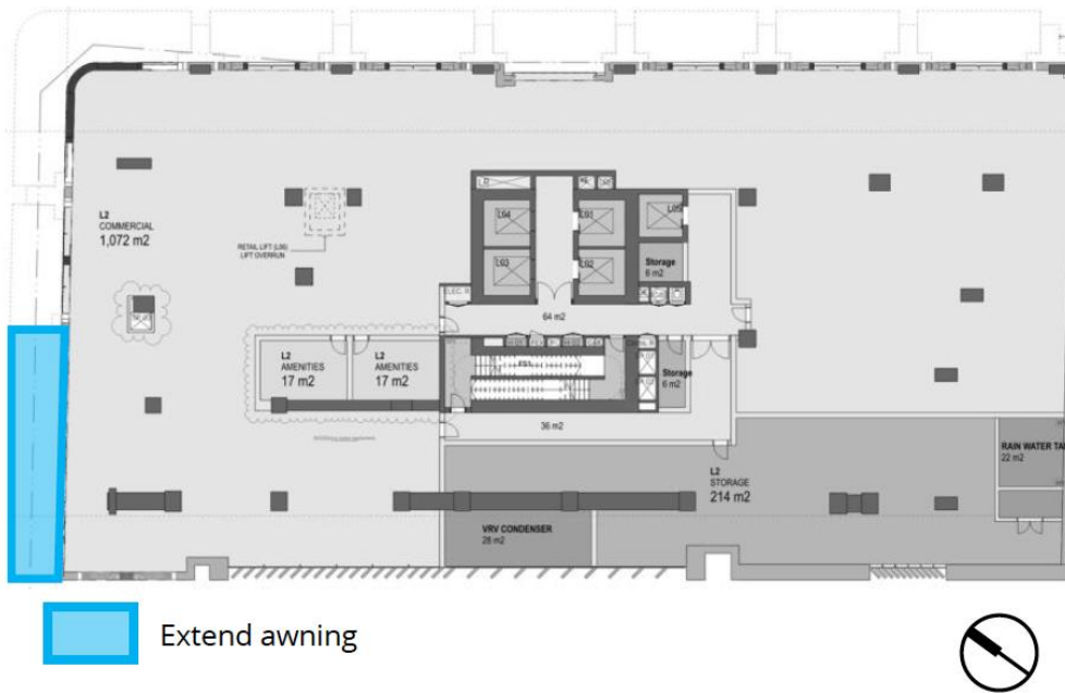
Figure 12: Podium level wind impact mitigation measures (Source: RWDI 2026)
