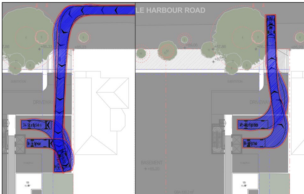
Figure 11 Swept path analysis – loading area
