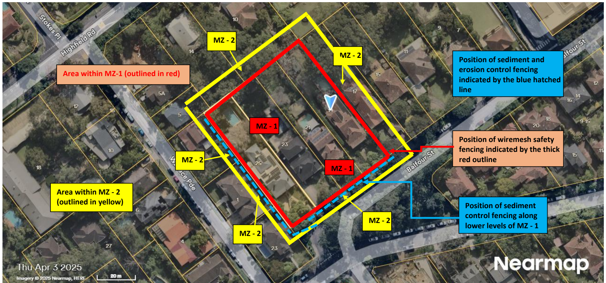
Figure 8 - Schematic representation of Management Zone delineation with sediment fence alignment (blue dashed lines) shown on an overlay from the aerial image on Nearmap (2025)
