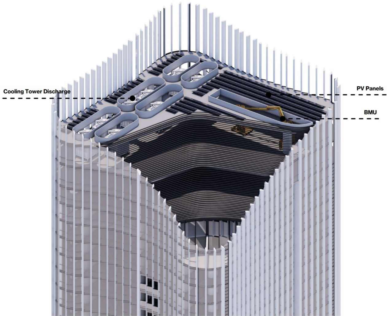
Figure 7 Tower Crown (illustrating the stepped nature of the roof form and plant zones over the height limit)
