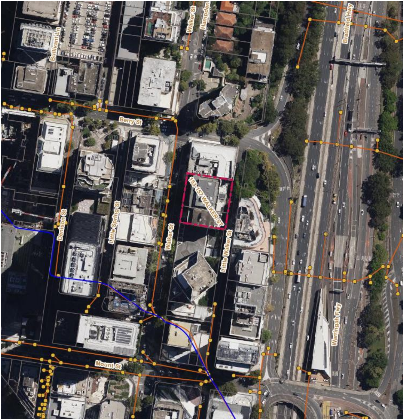
Figure 4: Existing Drainage Infrastructure from North Sydney Council Maps
