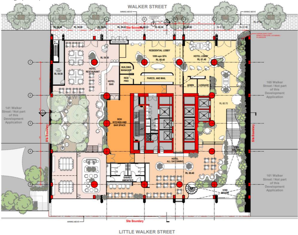
Figure 3 Architectural Plans – Ground Floor (residential and hotel lobbies, hotel bar, restaurant and all-day dining spaces)
