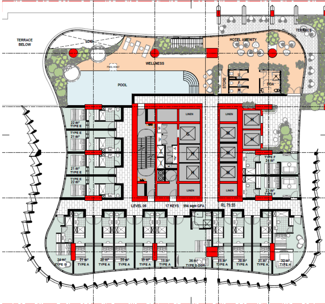
Figure 5 Architectural Plans - Level 6 (hotel floor and wellness space, pool and outdoor terrace)
