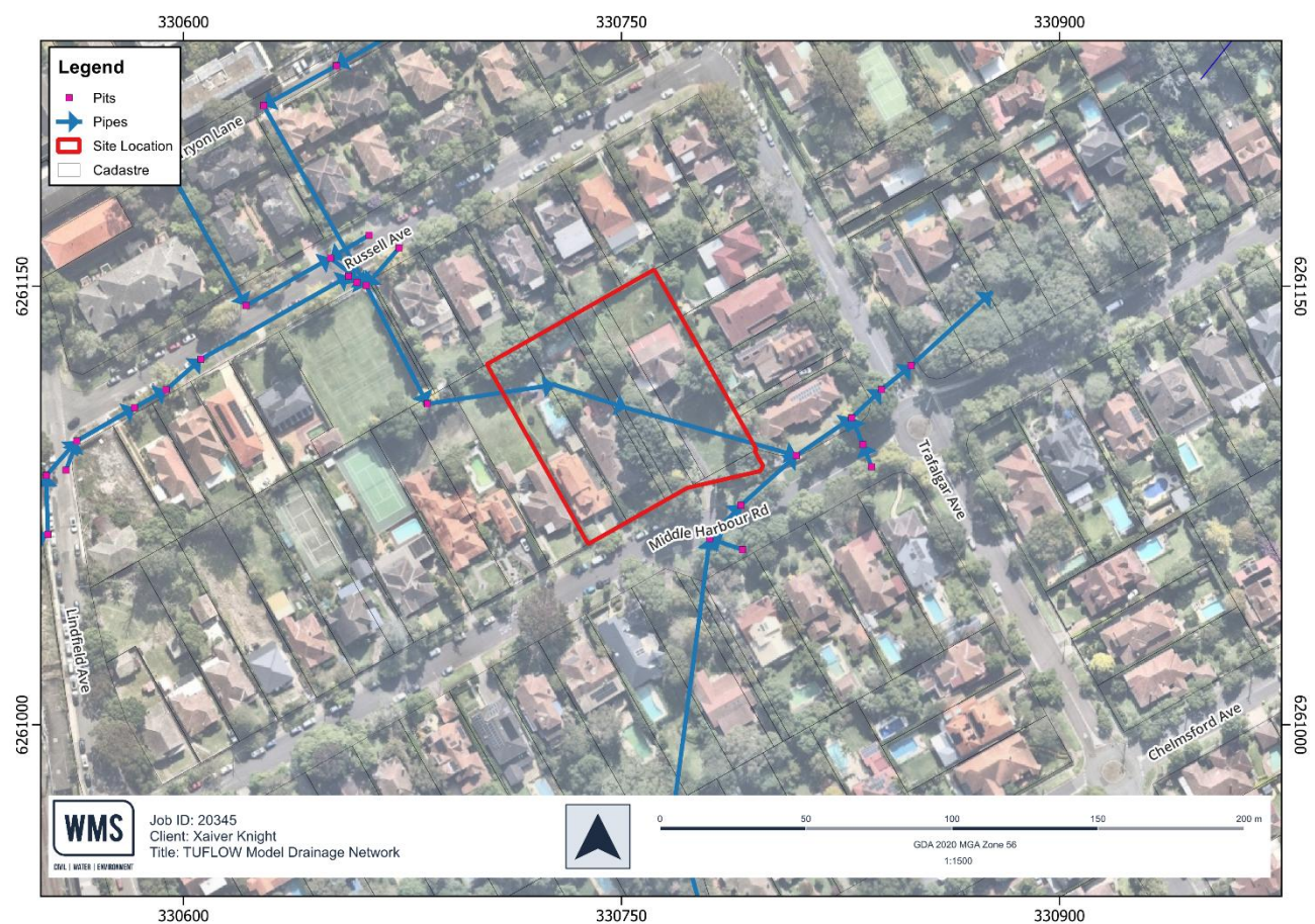
Figure 3-5 TUFLOW Model Drainage Network – Pre-Development
