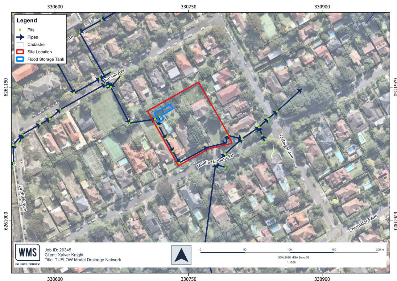
Figure 3-6 TUFLOW Model Drainage Network – Post-Development
