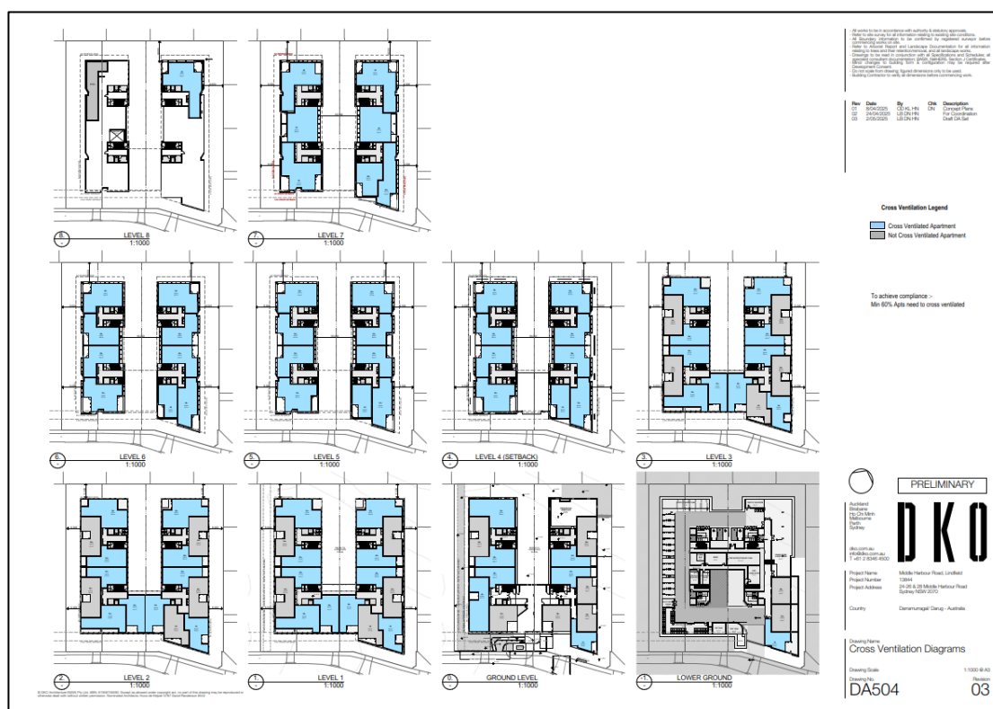
Figure 113. Cross Ventilation Diagrams.
