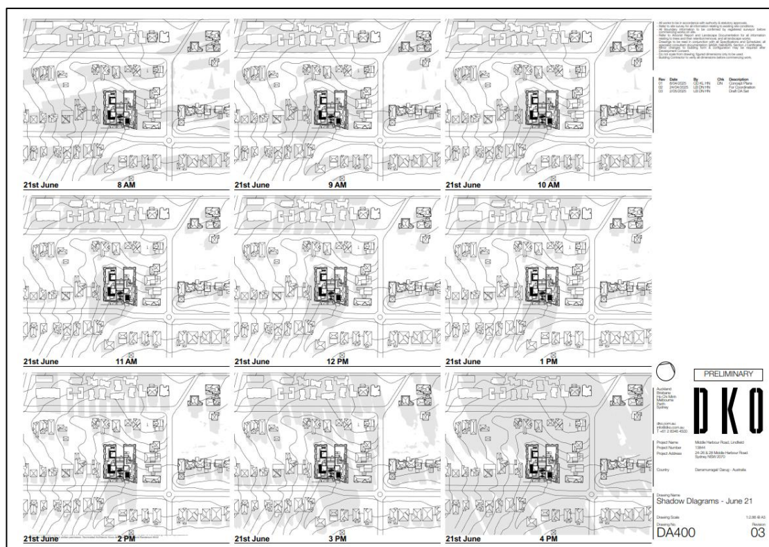
Figure 106. Shadow Diagrams – June 21.
