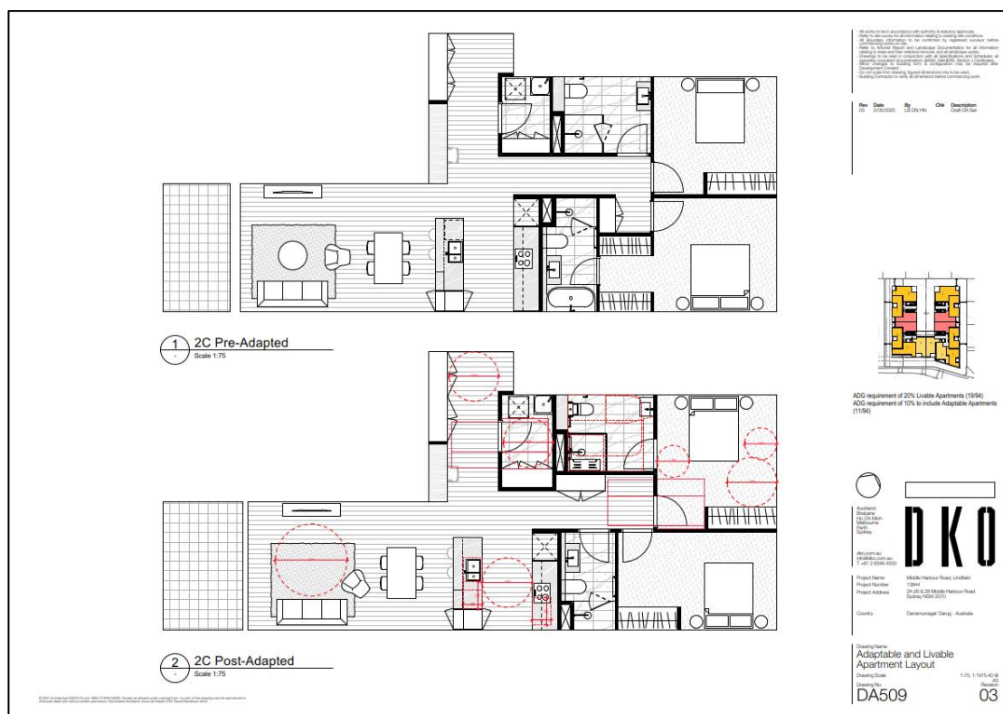
Figure 118. Adaptable and Liveable Apartment Layout.
